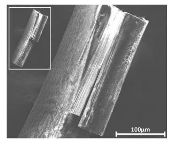
Fig. 3 Scanning Electron Microscope (SEM) image obtained using a high-resolution Hitachi \$4800 equipment (scale at the bottom right), showing the characteristic needle-like morphology of a small single crystal of synthetic nesquehonite, provided by the Yale Peabody Museum (specimen YPM MIN 031567). The sample was originally synthesized by Genth and Penfield<sup>21</sup> over a century ago. The inset shows the entire analyzed crystal.
