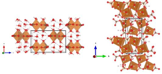
Fig. 2 Projection of MgCO<sub>3</sub>·3H<sub>2</sub>O nesquehonite along the b-axis (left) and a-axis (right) at room conditions. Magnesium (Mg), oxygen (O), carbon (C), and hydrogen (H) atoms are represented in orange, red, brown, and white, respectively.
