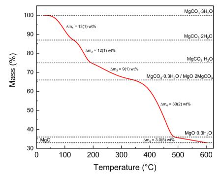
Fig. 4 Representative thermogravimetric model profile of nesquehonite based on literature-reported decomposition steps
