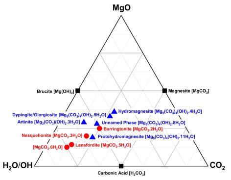
Fig. 1 Ternary diagram of the MgO-CO<sub>2</sub>-H<sub>2</sub>O system based on molar composition. Black squares represent the equimolar compounds found in the system, red circles indicate hydrated magnesium carbonates, and blue triangles denote basic magnesium carbonates.
