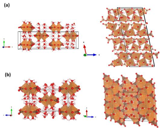
Fig. 6 (a) Crystal structure projections of the HP1 phase along the c-axis (left) and b-axis (right) at 3.1 GPa. (b) Crystal structure projections of the HP2 phase along the a-axis (left) and b-axis (right) at 11.6 GPa. Magnesium (Mg), oxygen (O), carbon (C), and hydrogen (H) atoms are shown in orange, red, brown, and white, respectively.
