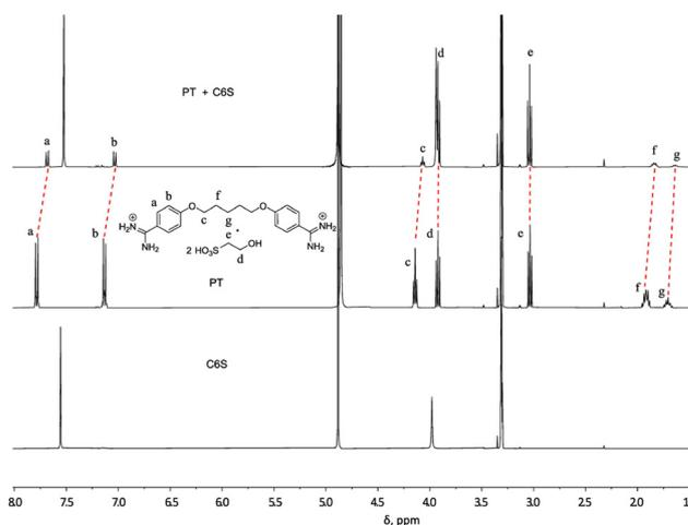
**Fig. 11** <sup>1</sup>H NMR spectra of C6S, pentamidine isethionate (PT) and host-guest complex – in the presence of some precipitate, recorded on an Agilent 400 MHz instrument at room temperature in CD<sub>3</sub>OD. *c*(C6S) = 4 mM, *c*(pentamidine) = 4 mM.
