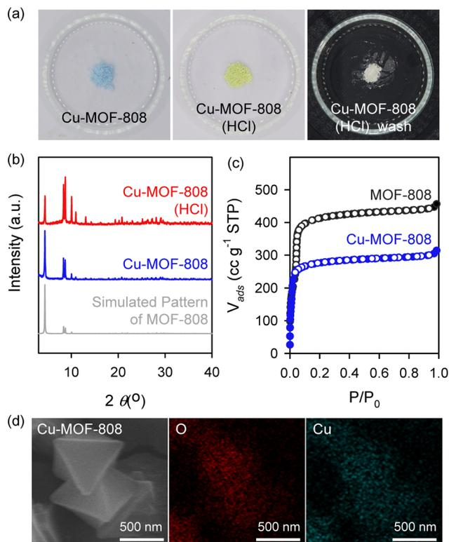
**Fig. 1** (a) Photographs of Cu-MOF-808 (left) and hydrochloric acid (HCl) exposed Cu-MOF-808 (centre), and Cu-MOF-808 exposed to HCl and subsequently washed with water (right). (b) XRPD patterns of Cu-MOF-808 (blue) and Cu-MOF-808 (HCl) (red) with simulated XRPD pattern of MOF-808 (grey). (c)  $\text{N}_2$  sorption isotherms of MOF-808 (black) and Cu-MOF-808 (blue) measured at 77 K. (d) SEM image (left) and EDS elemental mapping (centre and right) of Cu-MOF-808.
