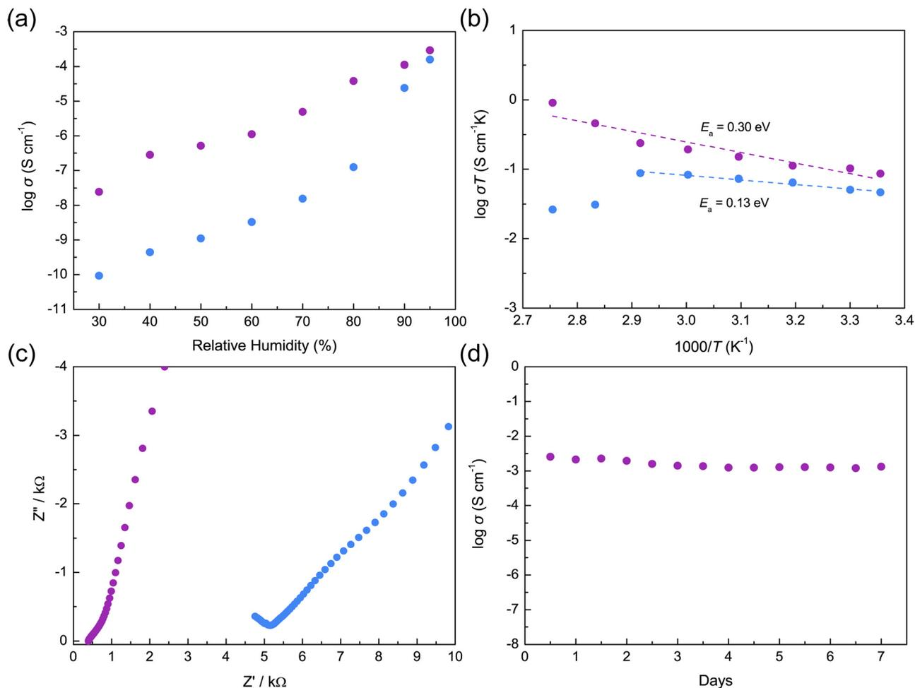
**Fig. 4** (a) Humidity-dependent conductivity of Y-DSNDC (blue) and K-DSNDC (purple) measured at 298 K. (b) Arrhenius plots for Y-DSNDC (blue) and K-DSNDC (purple) in the temperature range of 298–363 K under 95% RH. (c) Nyquist plots of the highest conductivity for Y-DSNDC (blue) and K-DSNDC (purple) measured at 343 K and 363 K under 95% RH, respectively. (d) Long-term stability of the proton conductivity for K-DSNDC at 363 K under 95% RH.
