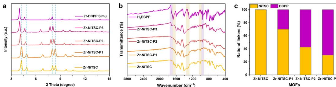
**Fig. 3** (a) PXRD patterns of Zr-NiTSC, Zr-NiTSC-P1, P2, and P3, and simulated non-interpenetrated Zr-DCPP, with blue vertical lines marking the low-angle shifting of diffraction peaks. (b) FT-IR spectra of Zr-NiTSC, Zr-NiTSC-P1, P2, and P3, and H<sub>2</sub>DCPP, with purple regions marking the increasing DCPD linkers and yellow regions marking the decreasing NiTSC linkers. (c) Ratio of NiTSC and DCPD linkers in Zr-NiTSC and Zr-NiTSC-P1, P2, and P3.
