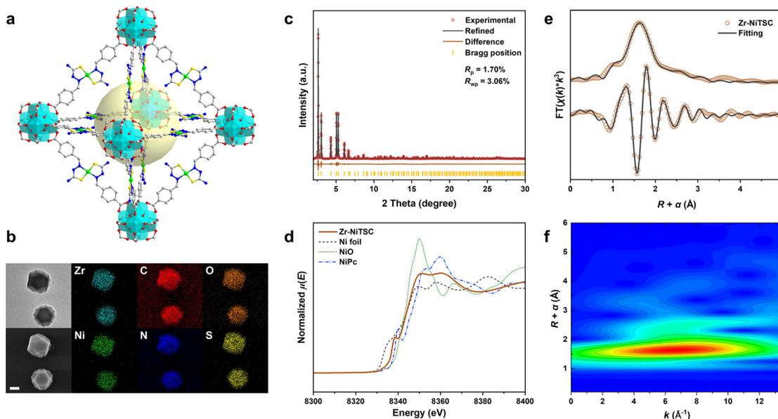
**Fig. 2** (a) Structure diagram of Zr-NiTSC. (b) TEM image, STEM image, and elemental mapping of Zr-NiTSC. Scale bar of 200 nm. (c) Pawley refinement of Zr-NiTSC (synchrotron PXRD,  $\lambda = 0.98 \text{ \AA}$ ). (d) Ni K-edge XANES spectra of Zr-NiTSC and standard samples Ni foil, NiO, and NiPc. (e) Ni K-edge EXAFS and the curfit for Zr-NiTSC, shown in  $R$ -space (FT magnitude and imaginary component). (f) Wavelet transform of  $\chi(k)$  of Zr-NiTSC.
