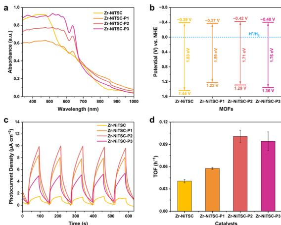
**Fig. 4** (a) Normalized UV-vis-NIR DRS spectra of Zr-NiTSC and Zr-NiTSC-P1, P2, and P3. (b) Band structure of Zr-NiTSC and Zr-NiTSC-P1, P2, and P3. (c) Transient photocurrent response of Zr-NiTSC and Zr-NiTSC-P1, P2, and P3. (d) TOFs of the Ni-N<sub>2</sub>S<sub>2</sub>-based photocatalysts.
