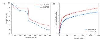
Fig. 3 (a) TG profiles and (b)  $\rm CO_2$  sorption isotherms obtained at 298 K for conv CALF-20 and mec CALF-20.
