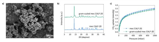
Fig. 4 (a) SEM image, (b) PXRD patterns, and (c) CO<sub>2</sub> adsorption isotherms of gram-scaled mec CALF-20 compared with mec CALF-20 at 298 K.
