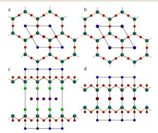
Fig. 1 Crystal structures of intercalates NH<sub>4</sub>Cl·As<sub>2</sub>O<sub>3</sub>·¹/<sub>2</sub>H<sub>2</sub>O (a and c) and NH<sub>4</sub>Br·2As<sub>2</sub>O<sub>3</sub> (b and d). Views along the crystallographic [001] (a and b) and [120] (c and d) directions. As, O, N, Cl, and Br atoms are depicted as teal, red, blue, light green and brown spheres, respectively. Violet spheres denote N and O atoms of disordered ammonium cations and water molecules. H atoms are omitted for clarity.
