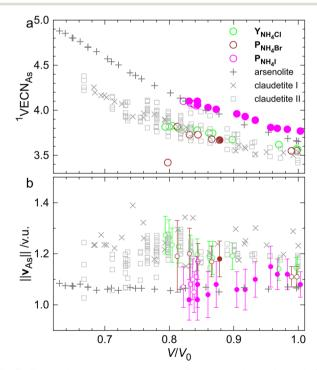
Fig. 5 First-order valence entropy coordination numbers of arsenic (a) and the magnitude of net BVV for arsenic (b) plotted as a function of the volume ratio  $V/V_0$  for the studied intercalates and for arsenic(III) oxide polymorphs. Data for arsenic(III) oxide polymorphs are taken from ref. 34–36.
