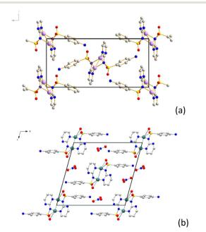
Fig. 5 Supramolecular packing of  $AgSD-NO_3$  depicting the formation of (a) chains along the *b*-axis and (b) the hexagonal array in the *a*-*c* plane.
