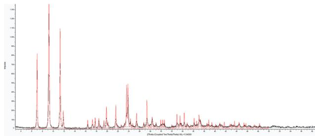
Fig. 4 PXRD of the new form AgSD-NO<sub>3</sub> (black) compared with the theoretical pattern (red).
