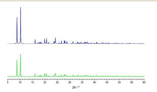
Fig. 2 PXRD diffractograms collected at  $\lambda$  (Cu K $\alpha_1$ ) = 1.54056 Å of AgSD reported as SULPMS (green) experimentally obtained by the LAG method and simulated (blue).
