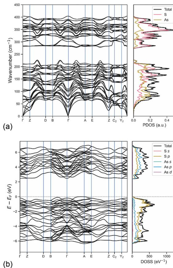
Fig. 6 Phonon and electronic properties of orpiment. (a) Phonon band structure and phonon density of states (PDOS) of bulk  $\text{As}_2\text{S}_3$  calculated at the DFT/B3LYP-D3 level of theory. (b) Electronic band structure and density of states (DOSS) of bulk orpiment  $\text{As}_2\text{S}_3$  obtained from DFT/HSE06-D3 simulations.
