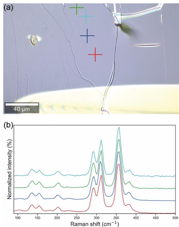
**Fig. 4** Confocal Raman microspectrometry analysis of an atomic-flat terrace of orpiment As<sub>2</sub>S<sub>3</sub>. (a) Optical microscopy image of the area investigated. (b) Raman spectra (excitation wavelength  $\lambda = 532$  nm) collected in the points marked with crosses in panel (a). The colours of the spectra match those of the markers in the optical image.
