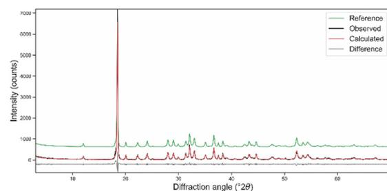
**Fig. 2** Powder diffraction data of orpiment  $As_2S_3$  and Rietveld refinement analysis. The difference between the calculated and measured intensities is reported below the profile. The reference XRPD pattern was taken from the American Mineralogist Crystal Structure Database #0010733, related to the sc-XRD data of Mullen and Nowacki.<sup>26</sup>
