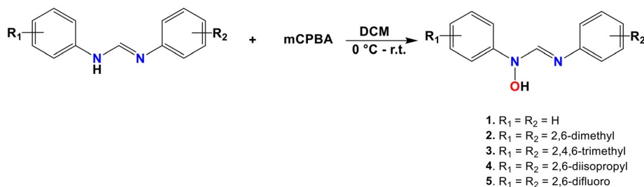
Scheme 1 Synthetic route to the formation of N -hydroxyformamidines.
