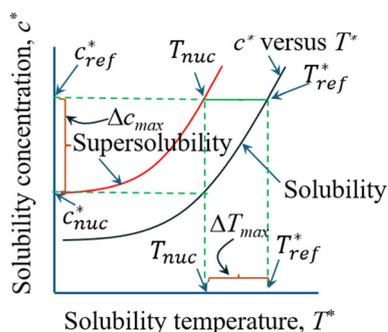
**Fig. 1** The relationship between solubility concentration,  $c^*$  and solubility temperature,  $T^*$ . Also shown in the figures are the different parameters that can be experimentally fixed or obtained and their relationship between the MSZW (or  $\Delta T_{\text{max}} = T_{\text{ref}}^* - T_{\text{nuc}}$ ) and the supersaturation (or  $\Delta c_{\text{max}} = c_{\text{ref}}^* - c_{\text{nuc}}^*$ ) at the MSZW.
