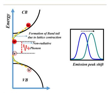
Fig. 17 Mechanism of shock wave-induced emission peak shift.
