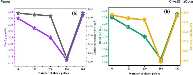
Fig. 14 Variation plot of bandgap, unit cell volume, and lattice parameters against a number of shock waves (a) bandgap vs. lattice parameters and (b) bandgap vs. unit cell volume.
