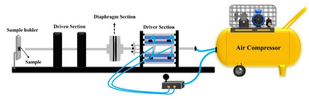
Fig. 1 The schematic representation of the semiautomatic Reddy tube.
