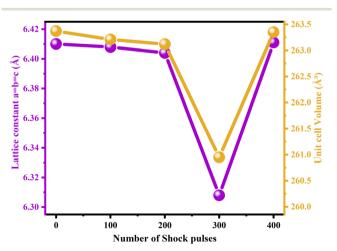
Fig. 8 The variation plot of lattice constant a = b = c (Å) and unit cell volume (Å<sup>3</sup>) against the number of shock pulses.
