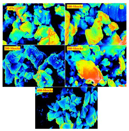
Fig. 20 2D surface profile of CdTe pre- and post-shock wave exposure.
