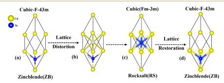
Fig. 6 Mechanism of reconstructable phase transition induced by acoustic shock wave from cubic-zincblende (ZB) to cubic-rocksalt (RS).
