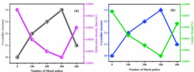
Fig. 9 The variation plots (a) crystallite size (nm) and dislocation density (lines per m<sup>2</sup>), (b) crystallite size (nm) and lattice strain (%) against the number of shock pulses.
