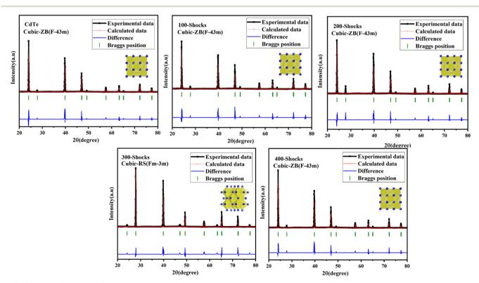
Fig. 7 Rietveld refinement of CdTe pre- and post-shock wave exposure.
