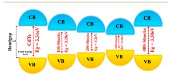
Fig. 15 Schematic representation of bandgap alignment of CdTe preand post-shock wave exposure.
