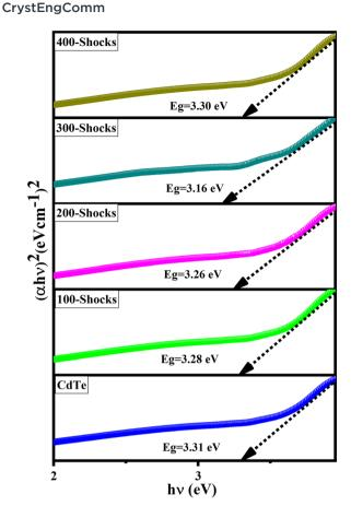
Fig. 12 Tauc plot of CdTe pre- and post-shock wave exposure.
