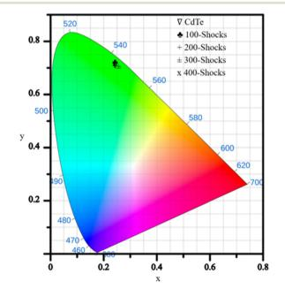
Fig. 18 CIE (x, y) chromaticity diagram of CdTe pre- and post-shock wave exposure.
