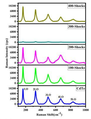
Fig. 10 Raman spectra of CdTe pre- and post-shock wave exposure.
