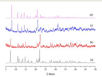
Fig. 12 (a) Simulated PXRD pattern of  $\bf 8$ , (b) PXRD pattern of the assynthesized  $\bf 8$ , (c) PXRD pattern of the sample of (b) heated in water at 100 °C for 2 days and (d) simulated PXRD pattern of  $\bf 9$ .
