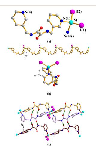
Fig. 3 (a) A representative drawing showing the coordination environment of the M(II) ion in 2-4. Symmetry transformations used to generate equivalent atoms: (A) 1 + x, 1 + y, 1 + z. (b) A drawing showing the 1D chain of 2-4. (c) A drawing showing the N-H···O hydrogen bonds.
