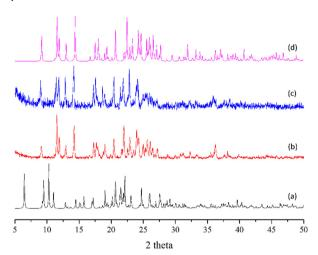
Fig. 11 (a) Simulated PXRD pattern of 1, (b) PXRD pattern of the assynthesized 1 exposed to air for five minutes, (c) PXRD pattern of the sample of (b) immersed in DMF and (d) simulated PXRD pattern of 2.
