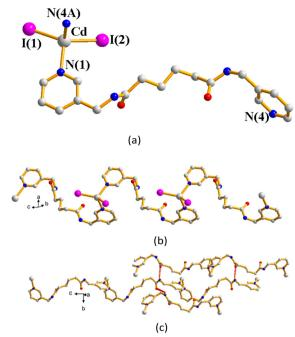
Fig. 6 (a) A drawing showing the coordination environment of the Cd(II) ion of 7. Symmetry transformations used to generate equivalent atoms: (A) -x, -y + 2, -z. (b) A drawing showing the 1D zigzag chain. (c) The 1D chains are linked through N-H···O hydrogen bonds.
