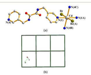
Fig. 8 (a) Coordination environment of Cd(II) in 9. Symmetry transformations used to generate equivalent atoms: (A) -x + 1, -y + 2, -z + 2; (B) x - 1, -y + 3/2, z + 1/2; (C) -x + 2, y + 1/2, -z + 3/2. (b) A drawing showing the structure of 9 with the sql topology.
