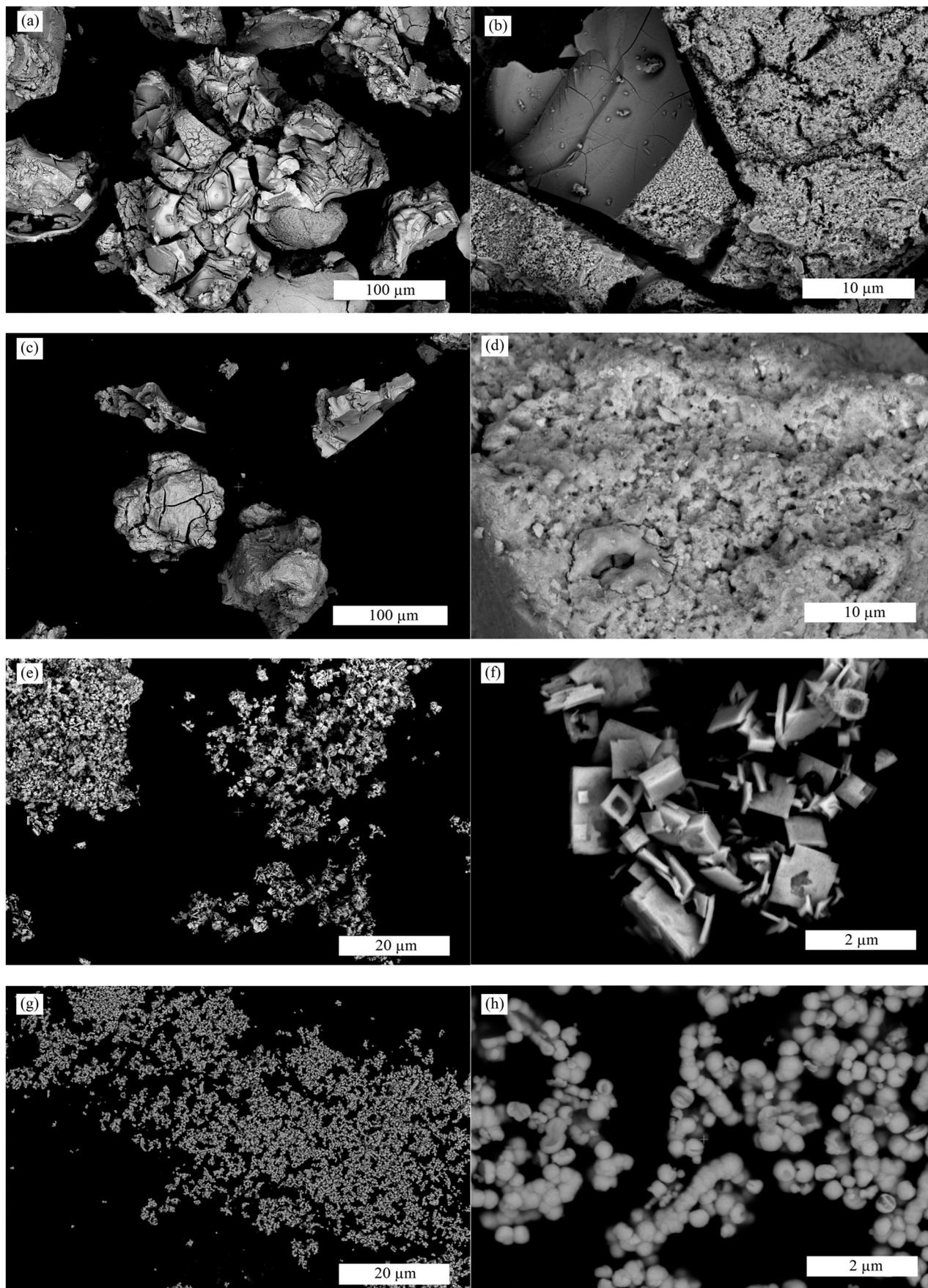
Fig. 2 SEM images of the ThO<sub>2</sub> powders obtained by different methods: HT (a) and (b); HH (c) and (d); OT (e) and (f); OH (g) and (h).
