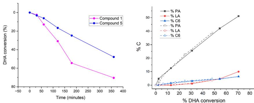
Fig. 4 DHA conversion (%) (left) and the identified resulting products (lactic acid (LA), pyruvaldehyde (PA) and C<sub>6</sub> sugars) for each test (right). Compound 1 (dinuclear Ta<sub>2</sub>O core): lines; compound 5 (octanuclear Ta<sub>8</sub>O<sub>12</sub> core): dash.
