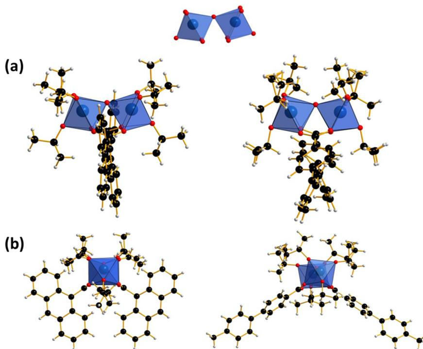
Fig. 1 Structural representation of compounds **1** and **2**; (a) side view showing the “*syn-syn*” bridging coordination mode and (b) top view illustrating the “*cis*” coordination of both carboxylate ligands.
