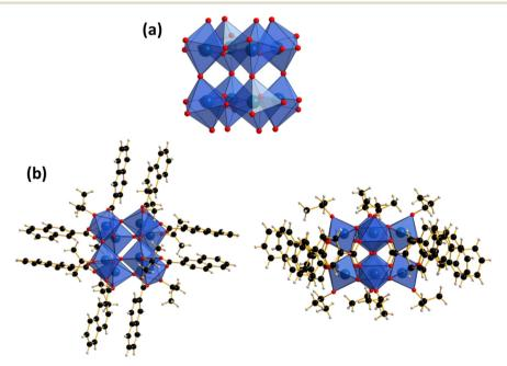
Fig. 3 Polyhedral representation of the molecular octanuclear coordination compound 5, [Ta<sub>8</sub>(μ-O)<sub>12</sub>(OiPr)<sub>8</sub>(C<sub>11</sub>H<sub>7</sub>O<sub>2</sub>)<sub>8</sub>]. (a) Nb-oxo core cluster and (b) top and side view of the complete octanuclear compound.
