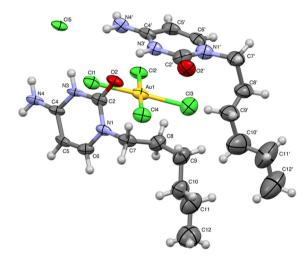
Fig. 5 View of asymmetric unit of X-ray structure for complex 2. The aliphatic chain of one cytosine is disordered and have been solved over two positions (C7A-C12A, 75% occupancy; C7C-C12C, 25% occupancy). The lower occupancy chain has been omitted for clarity.
