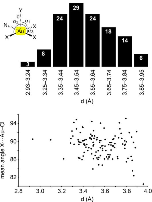
Fig. 13 Top: Histogram showing the distribution of CSD hits as a function of the  $\text{Y}\cdots\text{Au}$  distance. Bottom: Scatterplot of the mean  $\text{Y}\cdots\text{Au}-\text{Cl}$  angle ( $\alpha$ ) versus the  $\text{Y}\cdots\text{Au}$  distance.
