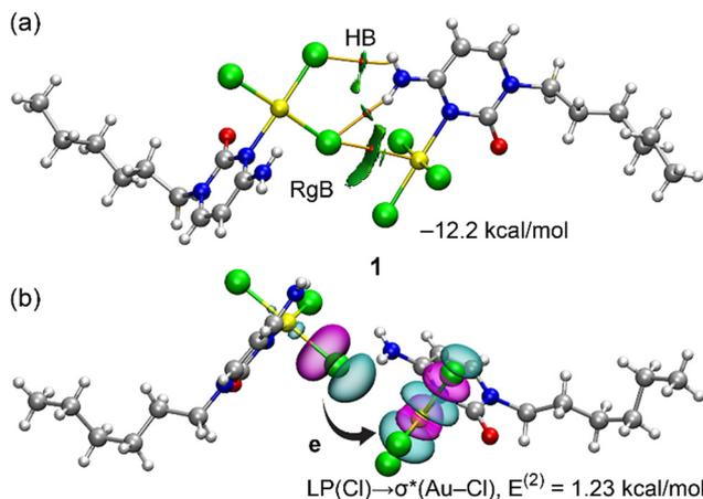
**Fig. 9** (a) Combined QTAIM (BCPs as red spheres and bond paths as orange lines) and NCIPLOT (RDG = 0.5,  $\rho$  cut-off = 0.04, color scale  $\pm 0.035$  a.u.) of the RgB dimer of **1**. Only intermolecular interactions are represented. The dimerization energies are indicated. (b) Donor and acceptors NBO corresponding to the  $\text{LP}(\text{Cl}) \rightarrow \sigma^*(\text{Au}-\text{Cl})$ . The second order perturbation energy is indicated.
