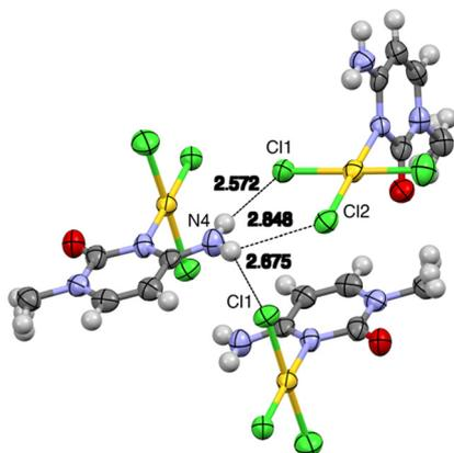
Fig. 3 View of hydrogen bond formed between the  $\text{NH}_2$  group and the chloride ligands in **1**. Distances in Å (aliphatic chains have been omitted for clarity). See Table 1 for  $\text{N}\cdots\text{Cl}$  distances with esd values.
