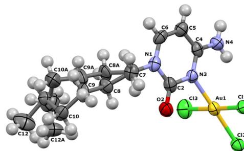
**Fig. 1** Asymmetric unit of complex AuCl<sub>3</sub>(CytC<sub>6</sub>). The aliphatic chain of the cytosine is disordered and have been solved over two equivalent (50% each) positions.
