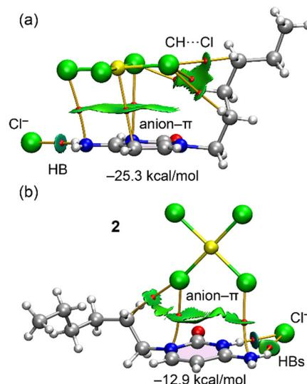
**Fig. 11** Combined QTAIM (BCPs as red spheres and bond paths as orange lines) and NCIPLOT (RDG = 0.5,  $\rho$  cut-off = 0.04, color scale  $\pm 0.035$  a.u.) for parallel (a) and T-shape (b) anion- $\pi$  binding modes. Only intermolecular interactions are represented.
