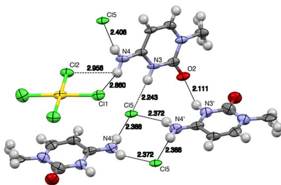
Fig. 7 View of the hydrogen bonds in the solid-state X-ray structure of complex 2. Distances in Å (aliphatic chains have been omitted for clarity). See Table 2 for the  $\text{N}\cdots\text{Cl}$  distances with esd values.
