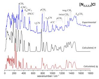
Fig. 4 INS spectrum of tetraethylammonium chloride, [N<sub>2,2,2,2</sub>]Cl (top line) and estimated INS intensities for two of its polymorphs: transtrans (middle line) and trans-gauche (bottom line). The assignments of some relevant vibrational modes are highlighted. Reproduced from ref. 34 with permission from the Royal Society of Chemistry.
