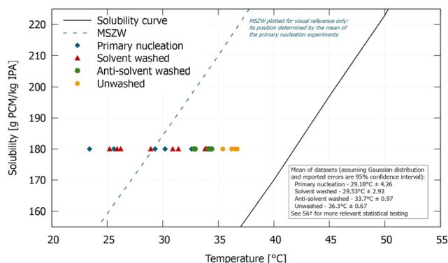
**Fig. 2** Impact of the selected washing procedure on the onset of nucleation. Only *solvent washed* is capable of fully eliminating initial breeding.
