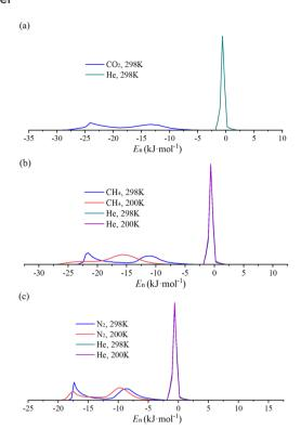
Fig. 6 Results of the adsorption energy distributions of  $CO_2$  and He at 298 K and 101 kPa (a);  $CH_4$  (b),  $N_2$  (c), and He in Cu-BTC at 298 K and 200 K. 101 kPa.
