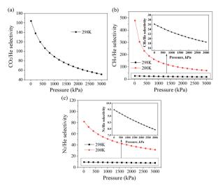
Fig. 3 The relationship between IAST selectivity coefficients and pressure for Cu-BTC at 298 K for CO<sub>2</sub>/He (50:50) (a), at 298 K and 200 K for  $CH_4/He$  (50:50) (b), and at 298 K and 200 K for  $N_2/He$ (50:50) (c) gas mixtures; pressure ranges from 0 to 3000 kPa.
