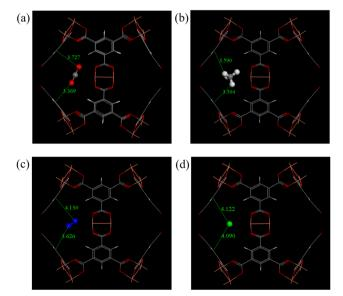
Fig. 7 The adsorption configurations of  $CO_2$  (a),  $CH_4$  (b),  $N_2$  (c), and He (d) at site A in Cu-BTC. Atomic colors: C (gray), O (red), N (blue), H (white), Cu (orange), He (green).
