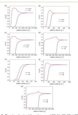
Fig. 8 The adsorption breakthrough curves of CO<sub>2</sub>/He (50:50) at 298 K (a),  $CH_4/He$  (50:50) at 298 K (b), 200 K (c), and 150 K (d), and  $N_2/He$ (50:50) at 298 K (e), 200 K (f), and 150 K (g) in Cu-BTC tested at a pressure of 101.324 kPa. The x-axis represents the ratio of time to sample mass, and the y-axis represents the ratio of the outlet to inlet concentration of the components.
