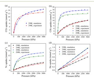
Fig. 2 Adsorption isotherm simulation and experimental results for CO<sub>2</sub> at 298 K (a), CH<sub>4</sub> at 298 K and 200 K (b), N<sub>2</sub> at 298 K and 200 K (c), and He at 298 K and 200 K (d) in Cu-BTC; pressure ranges from 0 to 3000 kPa.
