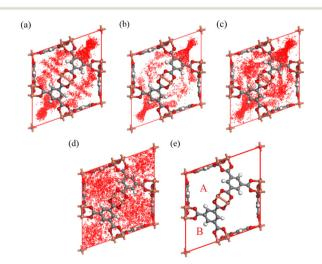
Fig. 5 Results of the density distributions of CO<sub>2</sub> (a), CH<sub>4</sub> (b), N<sub>2</sub> (c), and He (d) in Cu-BTC at 298 K and 101 kPa, along with a schematic diagram of the two adsorption sites in Cu-BTC (e).
