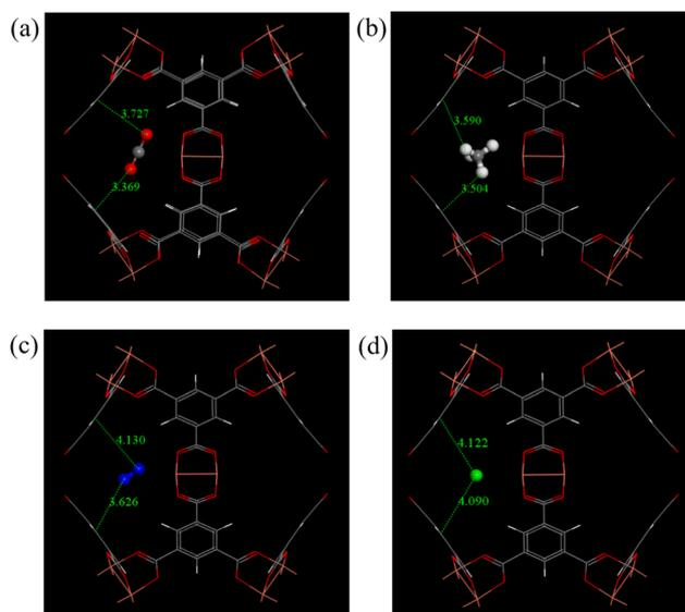
**Fig. 7** The adsorption configurations of CO<sub>2</sub> (a), CH<sub>4</sub> (b), N<sub>2</sub> (c), and He (d) at site A in Cu-BTC. Atomic colors: C (gray), O (red), N (blue), H (white), Cu (orange), He (green).
