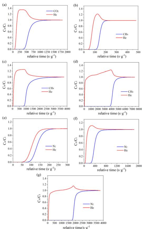
**Fig. 8** The adsorption breakthrough curves of CO<sub>2</sub>/He (50 : 50) at 298 K (a), CH<sub>4</sub>/He (50 : 50) at 298 K (b), 200 K (c), and 150 K (d), and N<sub>2</sub>/He (50 : 50) at 298 K (e), 200 K (f), and 150 K (g) in Cu-BTC tested at a pressure of 101.324 kPa. The x-axis represents the ratio of time to sample mass, and the y-axis represents the ratio of the outlet to inlet concentration of the components.
