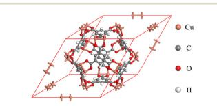
Fig. 1 Cu-BTC crystal structure.
