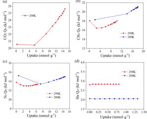
Fig. 4 Results of the heat of adsorption for CO<sub>2</sub> at 298 K (a), CH<sub>4</sub> at 298 K and 200 K (b), N2 at 298 K and 200 K (c), and He at 298 K and 200 K (d) in Cu-BTC.
