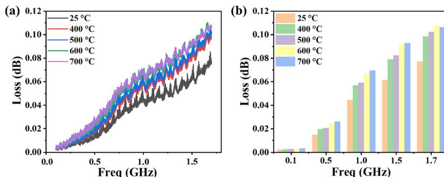
Fig. 6 (a) The relationship between the substrate loss of on-chip LiNbO<sub>3</sub> devices and frequency in the range of 0.1 to 1.7 GHz for untreated and treated samples at different reduction temperatures. (b) The substrate loss of on-chip LiNbO<sub>3</sub> devices at frequency points of 0.1 GHz, 0.5 GHz, 1.0 GHz, 1.5 GHz, and 1.7 GHz for untreated and treated samples at different reduction temperatures.
