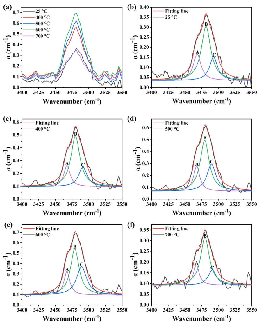
Fig. 4 (a) Infrared absorption spectra of LiNbO<sub>3</sub> untreated (25 °C) and treated at different reduction temperatures (400 °C, 500 °C, 600 °C, and 700 °C). Lorentzian multimodal fitting of the OH<sup>-</sup> IR absorption spectra for LiNbO<sub>3</sub> wafers (b) untreated (25 °C) and reduced at temperatures of (c) 400 °C, (d) 500 °C, (e) 600 °C, and (f) 700 °C.
