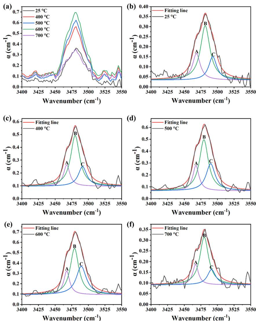
Fig. 4 (a) Infrared absorption spectra of LiNbO<sub>3</sub> untreated (25 °C) and treated at different reduction temperatures (400 °C, 500 °C, 600 °C, and 700 °C). Lorentzian multimodal fitting of the OH<sup>-</sup> IR absorption spectra for LiNbO<sub>3</sub> wafers (b) untreated (25 °C) and reduced at temperatures of (c) 400 °C, (d) 500 °C, (e) 600 °C, and (f) 700 °C.
