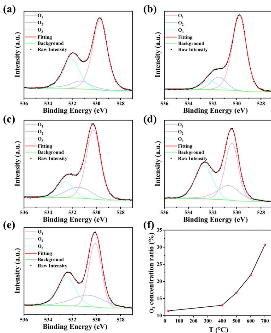
Fig. 5 (a) The O 1s electron spectra of  $\text{LiNbO}_3$  wafers untreated at 25 °C and treated at different reduction temperatures: (b) 400 °C, (c) 500 °C, (d) 600 °C, and (e) 700 °C, fitted using a Gaussian-Lorentzian mixed function. (f) Plot of the  $O_2$  concentration ratio on the surface of  $\text{LiNbO}_3$  crystals untreated at 25 °C and treated at different reduction temperatures (400 °C, 500 °C, 600 °C, and 700 °C).
