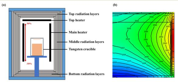
Fig. 1 (a) Schematic diagram of the interior of crystal growth (the red coordinate scale indicates the relative position of the seed crystal with respect to the center of the main heater). (b) The thermal field distribution within the crucible at 10% of the main heater's center position for the seed crystal.
