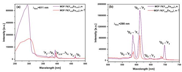
Fig. 14 (a) The excitation ( $\ell_{Emi} = 611$  nm) and (b) emission spectra ( $\ell_{Exc} = 290$  nm) of microcrystalline MOF-76( $Y_{0.95}$ Eu<sub>0.05</sub>)\_m and  $MOF-76(Y_{0.95}Eu_{0.05})_m-T.$
