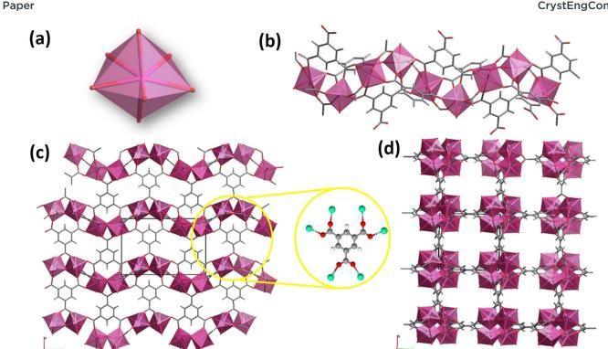
Fig. 2 (a) Coordination environment of  $Ln^{3+}$  ions in the MOF-76 structure. (b) Helical chains propagating along the c-axis. (c) View of the structure along the b-axis shows the six-connected nodes on BTC linkers in detail. (d) MOF-76 3D-structure showing cavities propagating along the c axis. DMF molecules were omitted for clarity.
