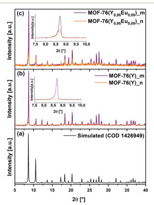
Fig. 1 Diffraction patterns of (a) Simulated MOF-76(Ho), (b) MOF- $76(Y)_m$  and MOF- $76(Y)_n$ , and (c) MOF- $76(Y_{0.95}Eu_{0.05})_m$  and MOF-76(Y<sub>0.95</sub>Eu<sub>0.05</sub>)\_n.
