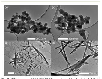
Fig. 7 TEM images of (a) MOF-76(Y)\_n sonicated for 5 min in EtOH. (b) MOF-76( $Y_{0.95}Eu_{0.05}$ )\_n sonicated for 5 min in EtOH. (c) MOF-76(Y)\_n sonicated for 15 min in H<sub>2</sub>O. (d) MOF-76(Y<sub>0.95</sub>Eu<sub>0.05</sub>)\_n sonicated for 15
