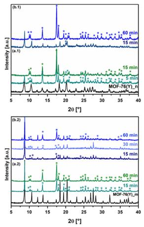
Fig. 4 MOF-76(Y)\_n in water: (a.1) sonicated, (b.1) non-sonicated. MOF-76(Y)\_m in water: (a.2) sonicated, (b.2) non-sonicated. All samples were not thermally activated for this experiment. The asterisk symbol over the peaks indicates the reflection of the 1D LnBTCcompound.
