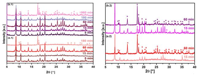
Fig. 10 MOF-76(Y)\_n in water: (a.1) sonicated, (b.1) non-sonicated. MOF-76(Y)\_m in water: (a.2) sonicated, (b.2) non-sonicated. All the samples were thermally activated for this experiment. The asterisk symbol over the peaks indicates the reflections of the LnBTC-compound.
