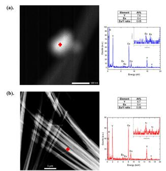
Fig. 8 STEM-HAADF image, point EDS spectrum, and calculated elemental composition of (a) one nanoparticle in MOF-76(Y<sub>0.95</sub>Eu<sub>0.05</sub>)\_n compound, and (b) MOF-76(Y<sub>0.95</sub>Eu<sub>0.05</sub>)\_n sonicated for 15 min in H<sub>2</sub>O. \*Copper signal comes from the TEM grid.
