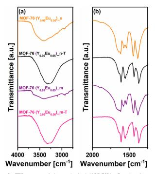
Fig. 9 FTIR spectra of the synthesized MOF-76(Y<sub>0.95</sub>Eu<sub>0.05</sub>)\_n (orange) compound and after sonication for 15 min in H<sub>2</sub>O (MOF-76(Y<sub>0.95</sub>Eu<sub>0.05</sub>)\_n-T, black), MOF-76( $Y_{0.95}Eu_{0.05}$ )\_m (purple) material and after sonication treatment for 60 min in  $H_2O$  (MOF-76( $Y_{0.95}Eu_{0.05}$ )\_m-T, pink), (a) from  $4000-2900 \text{ cm}^{-1} \text{ and (b) from } 2000-1250 \text{ cm}^{-1}$
