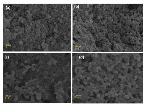
Fig. 11 SEM images of materials after activation: (a) MOF-76(Y)\_n as-synthesized form, (b) MOF-76(Y<sub>0.95</sub>Eu<sub>0.05</sub>)\_n as-synthesized form, (c) MOF-76(Y)\_n after thermal activation, and (d) MOF-76( $Y_{0.95}Eu_{0.05}$ )\_n after thermal activation.
