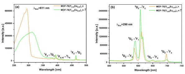
Fig. 15 (a) Excitation ( $\ell_{Emi}$  = 611 nm) and (b) emission spectra ( $\ell_{Exc}$  = 290 nm) of nanocrystalline MOF-76( $Y_{0.95}Eu_{0.05}$ )\_n compound and MOF-76( $Y_{0.95}Eu_{0.05}$ )\_n-T material.
