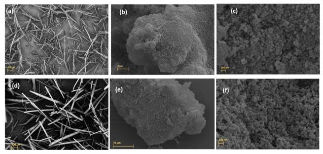
Fig. 3 SEM images of (a) MOF-76(Y)\_m needle-shape microcrystals. (b) Panoramic view of MOF-76(Y)\_n modulated by adding sodium acetate. (c)  $MOF-76(Y)_n$  showing the nanoparticles in detail. (d)  $MOF-76(Y_{0.95}Eu_{0.05})_n$  needle-shape microcrystals. (e)  $MOF-76(Y_{0.95}Eu_{0.05})_n$  modulated. (f) MOF-76(Y<sub>0.95</sub>Eu<sub>0.05</sub>)\_n nanoparticle.
