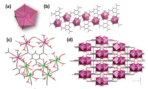
Fig. 6 (a) Coordination environment of  $Ln^{3+}$  ions in the LnBTC structure. (b) 1D ribbon-like structure along the *a* axis. (c) View of the carboxylate groups of coordination modes. (d) LnBTC framework.
