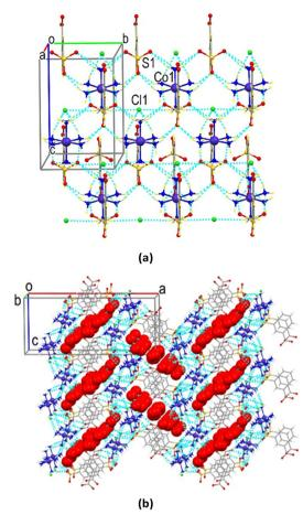
Fig. 3 (a) A fragment of the supramolecular layer in which the  $[\text{Co}(\text{NH}_3)_6]^{3+}$  cations are linked by H-bonds with the  $\text{Cl}^-$  anions and oxygen atoms of the sulfonate groups in 3. (b) Formation of channels in the crystal due to bridging of layers by N-H···O bonds of sulfonate and carboxylate groups of 3-sb. The solvent water molecules are shown in a space-filling mode, and hydrogen bonds are depicted as blue dashed lines.
