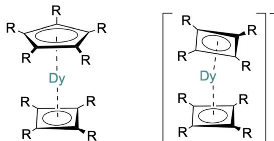
**Fig. 9** Future molecular design of high performance Dy-based SIMs of the general formula  $[\text{Dy}(\text{Cp}^{\text{R}})(\text{Cb}^{\text{R}})]$  (right) and  $\{\text{Dy}(\text{Cb}^{\text{R}})_2\}^-$  (left), where R is any alkyl, aryl, silyl, etc. group.
