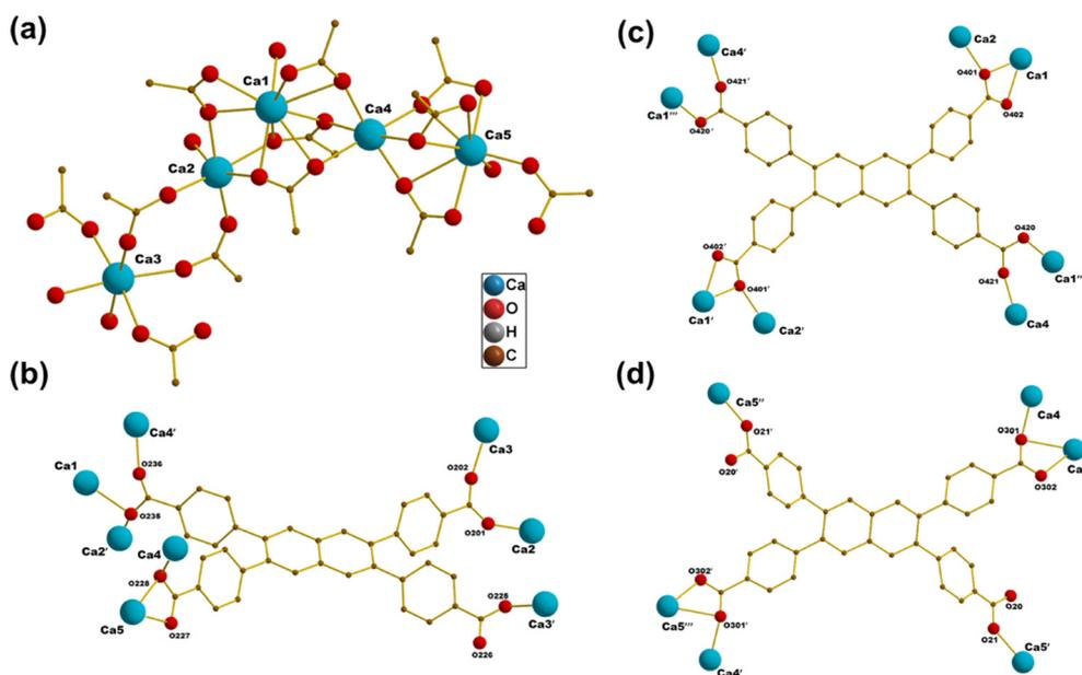
Fig. 9 (a): Coordination unit of the disrupted Ca chain in compound 3. (b) and (c): Coordination mode of the fully deprotonated  $\text{NTTB}^{4-}$  ligand. (d): Coordination mode of the partially deprotonated  $\text{H}_2\text{NTTB}^{2-}$  ligand.
