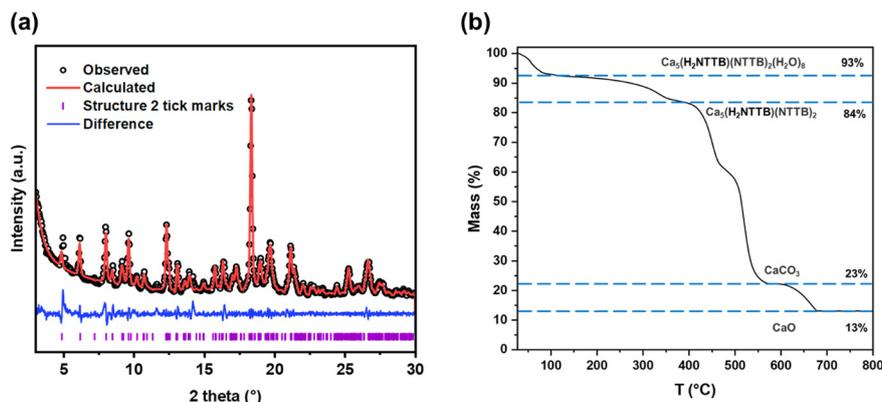
Fig. 7 (a) Pawley fit of powder XRD patterns of as-made sample of compound 2 ( $\text{Ca}_5(\text{H}_2\text{NTTB})(\text{NTTB})_2(\text{H}_2\text{O})_8$ ). The data points are shown in black, the fitted pattern in red, the difference curve in blue and the allowed tick positions in purple. The refined lattice parameters are shown in Table S1.† (b) Thermogravimetric analysis of compound 2 in air.
