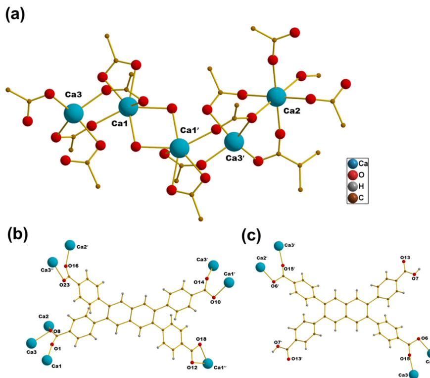
Fig. 6 (a) Local coordination of the Ca chain in compound 2. (b) Coordination mode of the fully deprotonated  $\text{NTTB}^{4-}$  ligand. (c) Coordination mode of the partially deprotonated  $\text{H}_2\text{NTTB}^{2-}$  ligand.
