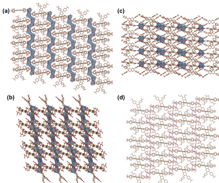
Fig. 5 Crystal structure of compound 2,  $\text{Ca}_5(\text{H}_2\text{NTTB})(\text{NTTB})_2(\text{H}_2\text{O})_6$ , viewed along *a* (a), *b* (b) and *c* (c) crystallographic axes. (d) Shows the simplified wireframe structure viewing along *a* axis.
