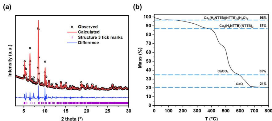
Fig. 10 (a) Pawley fit of powder XRD patterns of as-made sample of compound **3** ( $\text{Ca}_5(\text{H}_2\text{NTTB})(\text{NTTB})_2(\text{H}_2\text{O})_5$ ). The data points are shown in black, the fitted pattern in red, the difference curve in blue and the allowed tick positions in purple. (b) Thermogravimetric analysis in air of compound **3**.
