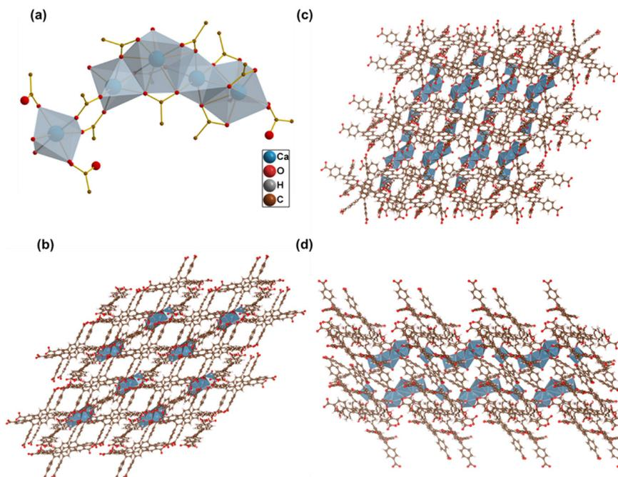
Fig. 8 Crystal structure of compound 3,  $\text{Ca}_5(\text{H}_2\text{NTTB})(\text{NTTB})_2(\text{H}_2\text{O})_5$ . (a):  $[(\text{Ca}_5)^{10+}]$  building unit. Structure viewed along a (b), b (c) and c (d) crystallographic axes.
