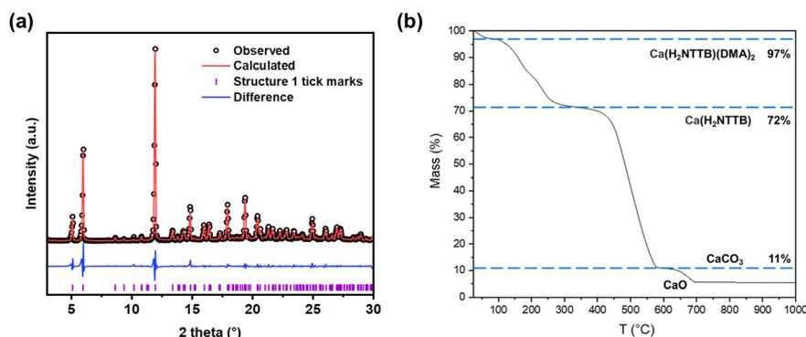
Fig. 4 (a) Pawley fit of powder XRD pattern of **1** ( $\text{Ca}(\text{H}_2\text{NTTB})(\text{DMA})_2$ ). The data points are shown in black, the fitted pattern in red, the difference curve in blue and the allowed tick positions in purple. The refined lattice parameters are shown in Table S1.† (b) Thermogravimetric analysis of compound **1** in air.
