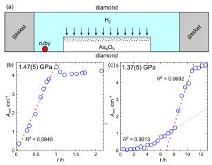
Fig. 7 Schematic drawing of the applied experimental setup; note that proportions between different parts in the drawing are not maintained (a). The peak area of inclusion compound As<sub>4</sub>O<sub>6</sub>·2H<sub>2</sub> plotted as a function of time for the peak around 250 cm<sup>-1</sup>. Measurements were carried out at 1.47 (5) and 1.37 (5) GPa (b and c, respectively). Figure adapted from P. A. Guńka, K. F. Dziubek and F. Capitani, J. Phys. Chem. C, 2023, 127, 15871-15875.21
