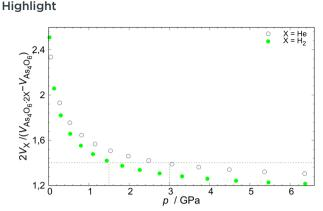
Fig. 5 The ratio of hydrogen or helium molar volumes to the difference between molar volumes of arsenolite and its inclusion compound with hydrogen or helium plotted as a function of pressure.  $X = H_2$ , He. Reprinted with permission from P. A. Guńka, M. Hapka, M. Hanfland, G. Chałasiński and J. Zachara, *J. Phys. Chem. C*, 2019, **123**, 16868–16872. <sup>19</sup> Copyright 2019 American Chemical Society.
