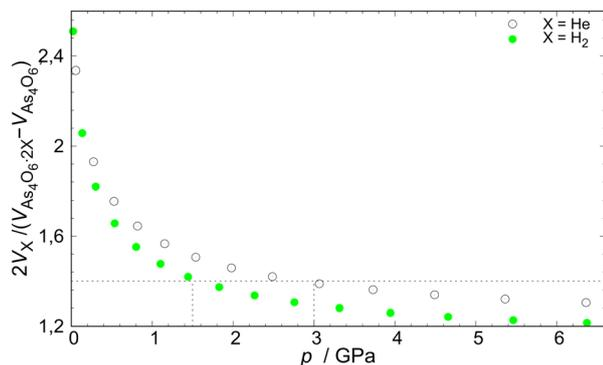
Fig. 5 The ratio of hydrogen or helium molar volumes to the difference between molar volumes of arsenolite and its inclusion compound with hydrogen or helium plotted as a function of pressure. X = H<sub>2</sub>, He. Reprinted with permission from P. A. Guńka, M. Hapka, M. Hanfland, G. Chataśiński and J. Zachara, *J. Phys. Chem. C*, 2019, **123**, 16868–16872.<sup>19</sup> Copyright 2019 American Chemical Society.
