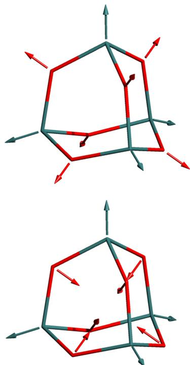
Fig. 2 The molecular structure of  $\text{As}_4\text{O}_6$  presented in the wireframe model and symmetry coordinates of molecular deformations: scaling  $\zeta$  (top) and distortion  $\eta$  (bottom). Arsenic and oxygen atoms denoted green and red, respectively.
