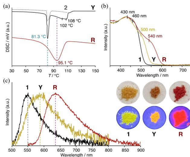
**Fig. 5** a) DSC traces showing the thermal behavior of Y, R, and pure naphthalene (2) with increasing temperature. Solid-state b) absorption and c) emission spectra of Y, R, and the empty crystal of 1. On the right, the top and bottom photos show the absorption colors under room light and the emission colors under UV irradiation (375 nm), respectively.
