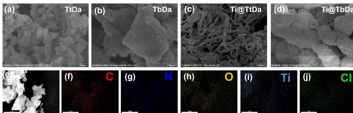
Fig. 2 SEM image of the parent COF and Ti@COF. SEM images of (a) TtDa, (b) TbDa, (c) Ti@TtDa, and (d) Ti@TbDa. (e)-(j) The EDX-mapping images of Ti@TtDa.
