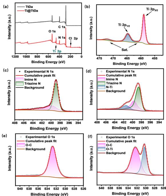
**Fig. 3** XPS analysis of TtDa and Ti@TtDa. (a) Survey spectra of TtDa and Ti@TtDa; (b) high-resolution Ti 2p spectrum of Ti@TtDa; (c) high-resolution N 1s spectrum of TtDa; (d) high-resolution N 1s spectrum of Ti@TtDa; (e) high-resolution O 1s spectrum of TtDa; (f) high-resolution O 1s spectrum of Ti@TtDa.
