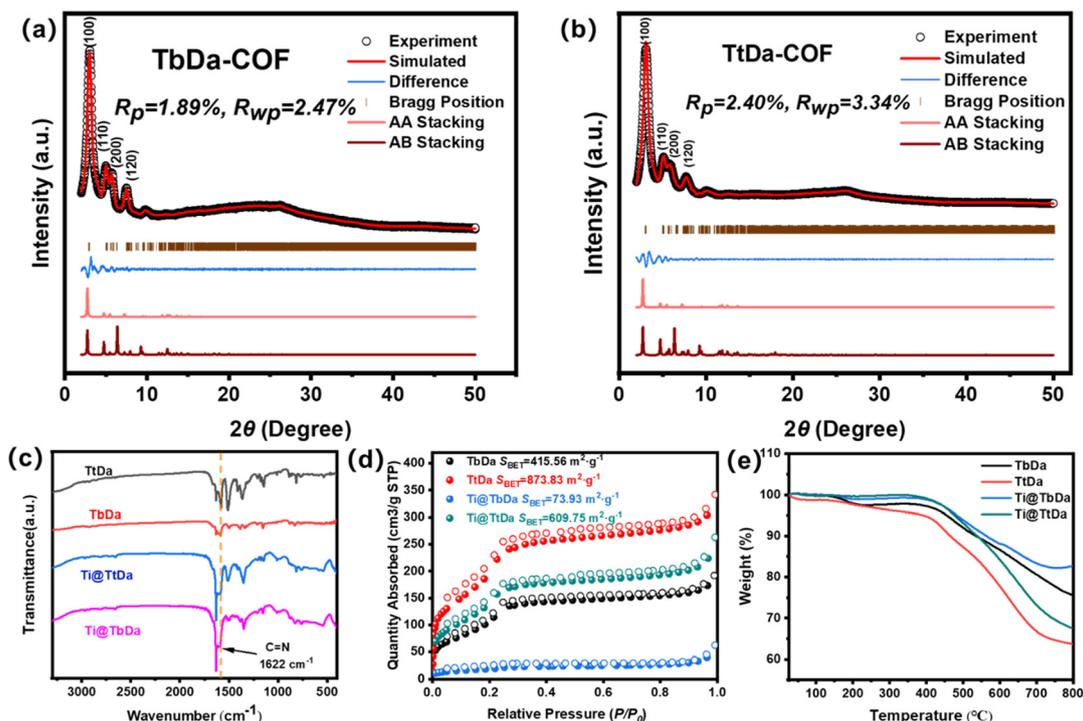
Fig. 1 The experimental and Pawley refined predicted powder X-ray diffraction (PXRD) patterns of TbDa (a) and TtDa (b); the infrared spectra of TbDa, TtDa, Ti@TbDa, and Ti@TtDa (c), the  $\text{N}_2$  adsorption-desorption isotherms (d), and TGA curves under an  $\text{N}_2$  atmosphere (e).
