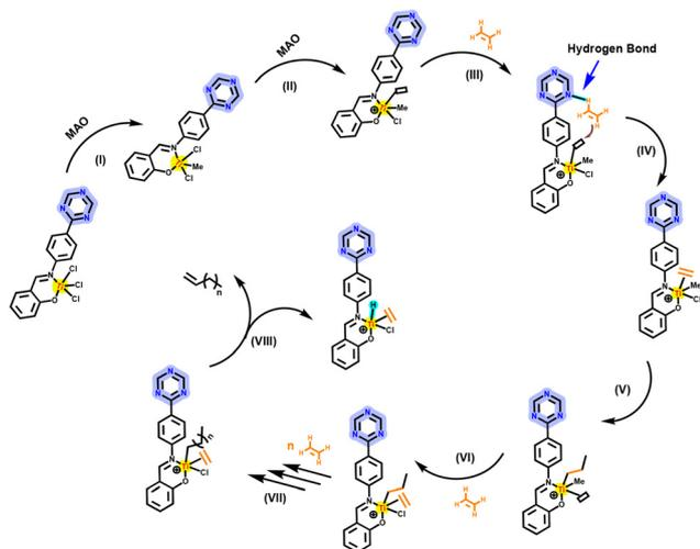
**Scheme 2** Ti@TtDa ethylene polymerization mechanism under a low ethylene pressure (note: steps I to III are the chain initiation processes, steps IV to VII are the chain growth processes, and step VIII is the chain termination process).
