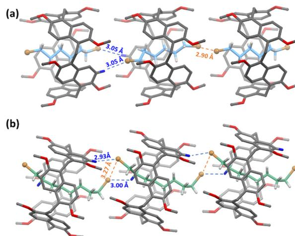
Fig. 4 Crystal structures of the linear supramolecular polymer backbone driven by the guest in the inclusion complexes of [PS-5  $\supset$  DBH] (a) and the higher occupancy guest conformation in [PS-5  $\supset$  DBO] (b).
