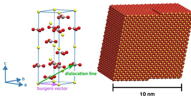
**Fig. 1** Left: Unit cell of the calcite crystal and illustration of the dislocation line and the Burgers vector imposed to create the screw-like structure from the single crystal. Right: Simulation model of the calcite crystallite featuring the (104), (014) and (114) surfaces. Note that the chosen shape and the mixed dislocation results in a smooth structure, which is stable in both vapor and water.
