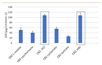
Fig. 2 IDR for the salts of CBZ at a pH of 6.8
