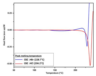
Fig. 4 DSC thermograms of the CBZ·HBr and CBZ·HCl salts.
