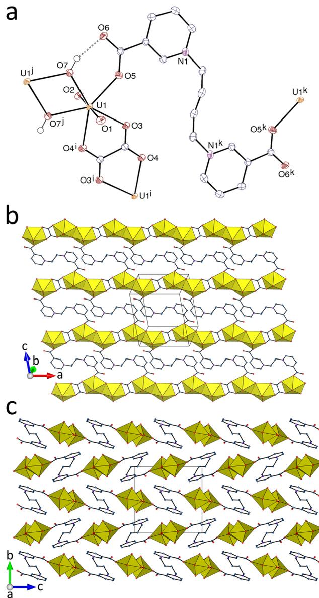
**Fig. 4** (a) View of compound 4 with displacement ellipsoids shown at the 50% probability level. Carbon-bound hydrogen atoms are omitted and the hydrogen bond is shown as a dashed line. Symmetry codes:  $i = 1 - x, 1 - y, -z$ ;  $j = 2 - x, 1 - y, -z$ ;  $k = 1 - x, 1 - y, 1 - z$ . (b) The diperiodic coordination polymer. (c) Packing with layers viewed edge-on.
