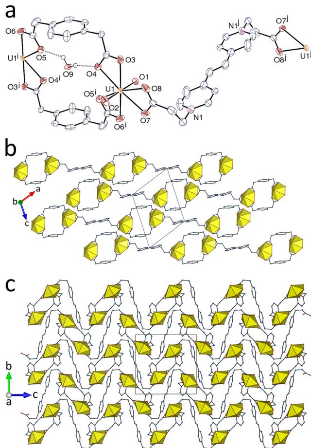
**Fig. 2** (a) View of complex **2** with displacement ellipsoids shown at the 50% probability level. Carbon-bound hydrogen atoms are omitted and hydrogen bonds are shown as dashed lines. Symmetry codes:  $i = -x, 1 - y, 1 - z$ ;  $j = 2 - x, 1 - y, 2 - z$ . (b) Arrangement of monoperic coordination polymers parallel to (010). (c) Packing with chains viewed edge-on.
