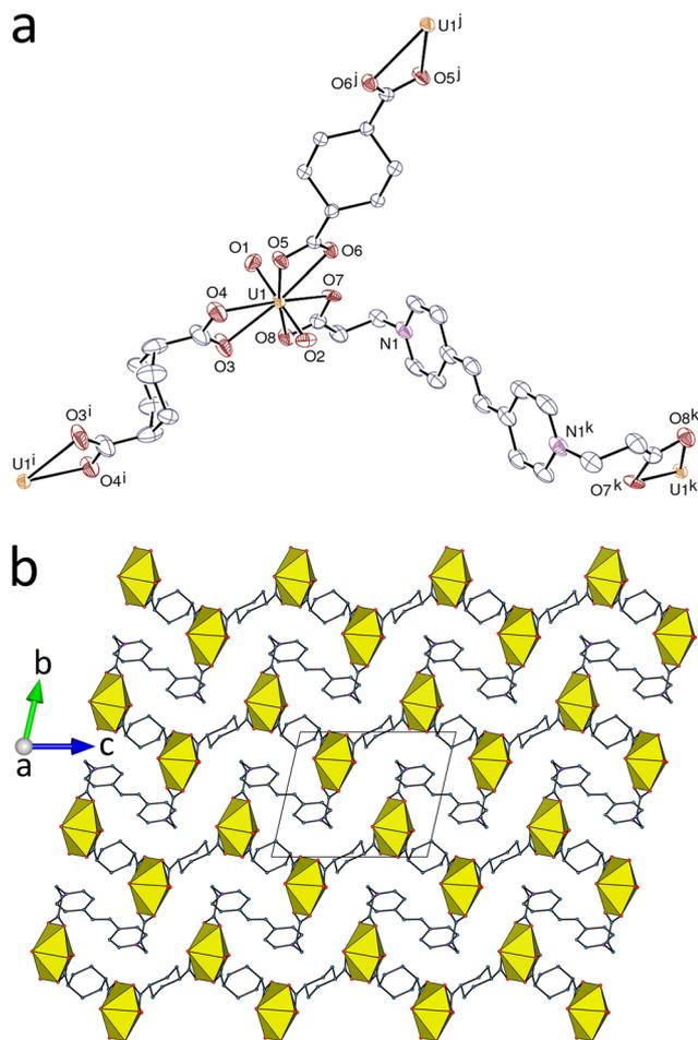
**Fig. 3** (a) View of compound 3 with displacement ellipsoids shown at the 40% probability level and hydrogen atoms omitted. Symmetry codes:  $i = 2 - x, 2 - y, -z$ ;  $j = -x, 2 - y, 1 - z$ ;  $k = -x, 1 - y, -z$ . (b) View of the hcb diperiodic coordination polymer.
