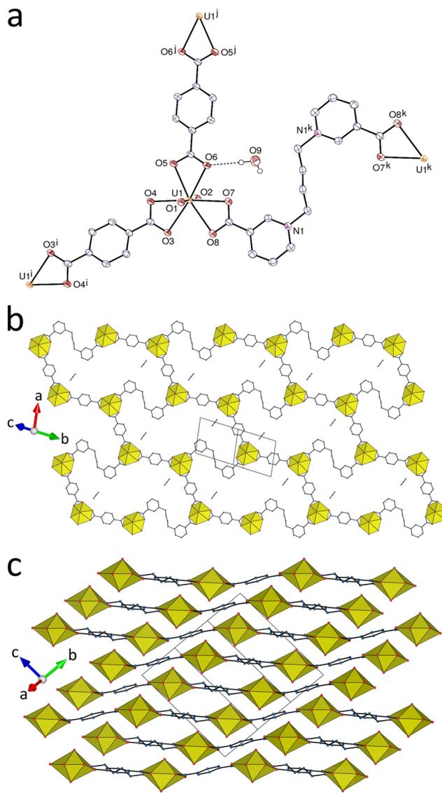
**Fig. 6** (a) View of compound 6 with displacement ellipsoids shown at the 50% probability level. Carbon-bound hydrogen atoms are omitted and the hydrogen bond is shown as a dashed line. Symmetry codes:  $i = 1 - x, 2 - y, -z$ ;  $j = 2 - x, 1 - y, 1 - z$ ;  $k = -x, -y, 1 - z$ . (b) View of the **hcb** diphasic coordination polymer with included acetonitrile molecules. (c) Packing with layers viewed edge-on and solvent excluded.
