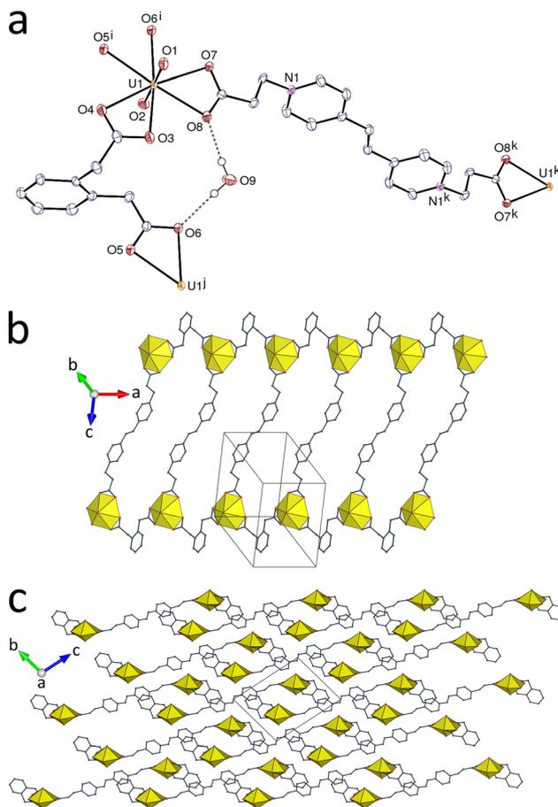
Fig. 1 (a) View of complex **1** with displacement ellipsoids shown at the 50% probability level. Carbon-bound hydrogen atoms are omitted and hydrogen bonds are shown as dashed lines. Symmetry codes:  $i = x - 1, y, z$ ;  $j = x + 1, y, z$ ;  $k = 1 - x, 2 - y, -z$ . (b) The two-stranded monoperoic coordination polymer with uranium coordination polyhedra in yellow. (c) Packing with chains viewed end-on.
