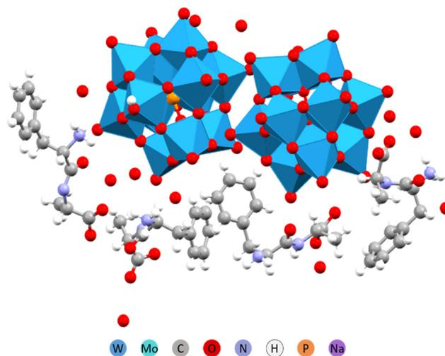
Fig. 7 Molecular structure of the  $(\text{H}_3\text{O})_2(\text{HPhe-Ala})_4[\text{PW}_{12}\text{O}_{40}]_2\cdot 11\text{H}_2\text{O}$ .<sup>32</sup>
