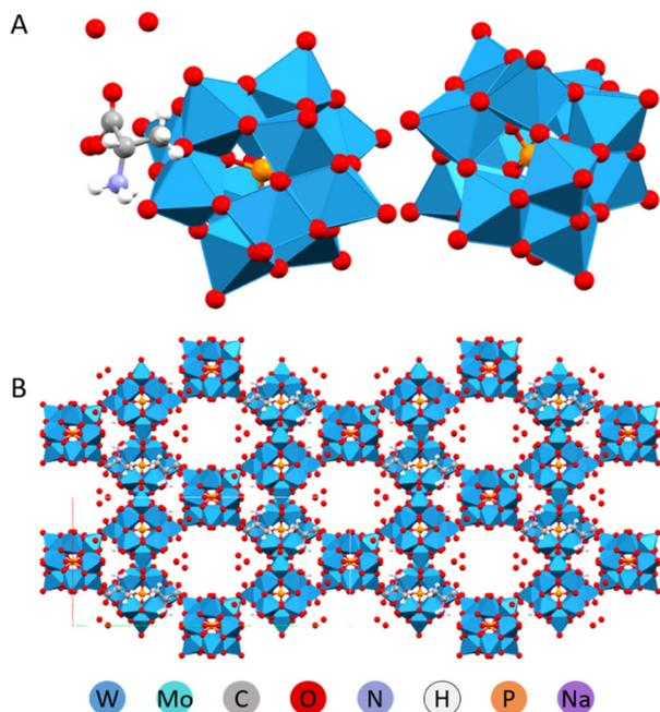
Fig. 10 Molecular (A) and crystal (B) structure of the (HAla) $H_5[PW_{12}O_{40}]_2 \cdot 4H_2O$ .<sup>33</sup>
