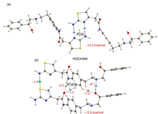
Fig. 11 Overlapped QTAIM and NCIplot analyses of the  $R_2^2(8)$  synthon (a) and head-to-tail infinite chains (b) in dimers of mirabegron (HOCHAM). The energies of the synthons are given in kcal mol<sup>-1</sup>.
