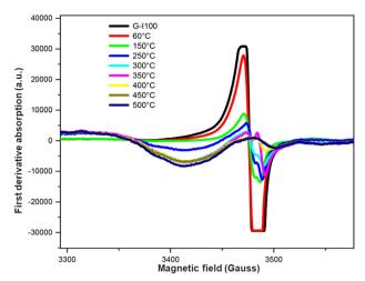
Fig. 8 EPR spectra for G-I100 before the annealing treatment and after annealing (G-IA100) at temperatures between 60 and 500  $^{\circ}$ C.
