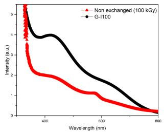
Fig. 4 Optical absorption spectra of the non-exchanged glass (red curve) and the Cu-exchanged glass (black curve) after being irradiated at 100 kGv.
