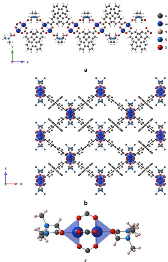
**Fig. 2** Portion of the X-ray structure for **1** showing the formation of the 2D neutral coordination network resulting from the bridging of the consecutive ligand **L** by Cu<sup>2+</sup> cations: a) view of the corrugated plane along the *b* axis, b) view of the grid in the *xOz* plane c) details of the environment around Cu<sup>2+</sup> cations. H atoms are not all presented for clarity. Disordered DMF molecules are represented.
