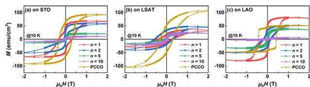
**Fig. 4** Magnetic-field dependence of the magnetization curves of the  $(\text{PCO})_n/(\text{CCO})_n$  SLs and PCCO films measured at 10 K on the (a) (001) STO, (b) (001) LSAT, and (c) (001) LAO substrates, respectively. For easy comparison, (a) is replotted from ref. 22.
