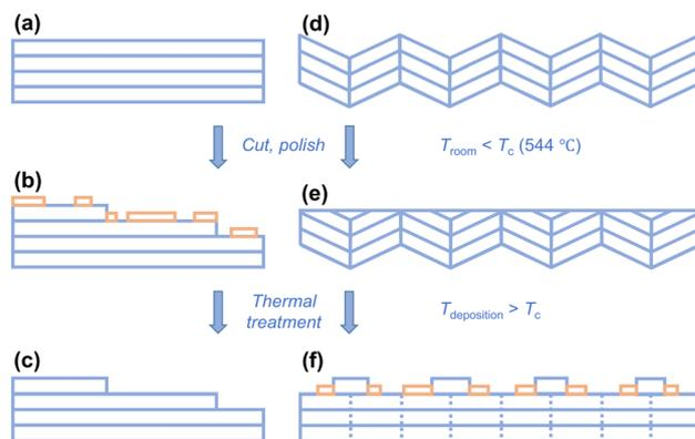
Fig. 3 The evolution of different substrate surface structures. (a)–(c) The surface-step-terrace structure on the STO substrate. (d)–(f) The twinned zig-zag facet structure on the LAO substrate.  $T_c$  is the phase transition temperature (544 °C) of LAO from the pseudocubic rhombohedral  $R\bar{3}c$  phase to the cubic  $Pm\bar{3}m$  phase.
