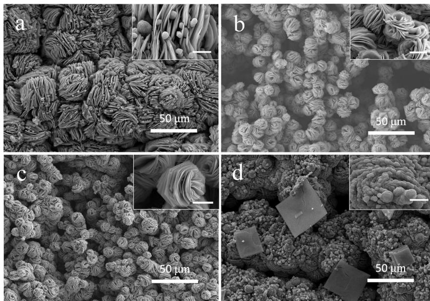
Fig. 2 SEM micrographs of  $\text{VS}_2/\text{SS}$  prepared with different molar ratios of  $\text{NH}_4\text{VO}_3$ :TAA (a) 1:2.5 (b) 1:5 (c) 1:7.5 (d) 3:5 (the scale bar in the inset images is 5  $\mu\text{m}$ ).
