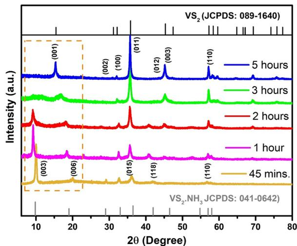
Fig. 8 XRD patterns of VS<sub>2</sub>/SS hydrothermally synthesized with different reaction times (45 min, 1, 2, 3, and 5 hours).
