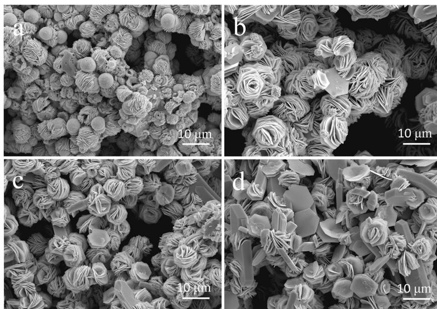
Fig. 10 (a–d) SEM micrographs of VS<sub>2</sub>/SS synthesized by adding 0 mL, 2 mL, 4 mL, and 6 mL of ammonia solution in the reaction vessel during the hydrothermal reaction.
