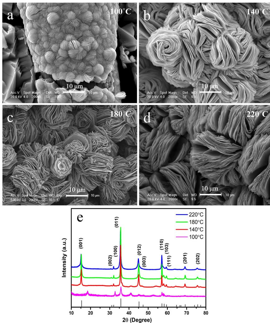
Fig. 5 (a–d) SEM images and (e) XRD patterns of VS<sub>2</sub>/SS samples synthesized at different reaction temperatures of 100 °C, 140 °C, 180 °C, and 220 °C for 20 hours of heating time. The molar ratio of NH<sub>4</sub>VO<sub>3</sub> and TAA was 1:7.5 in mmol, while their mass loading was 3×.
