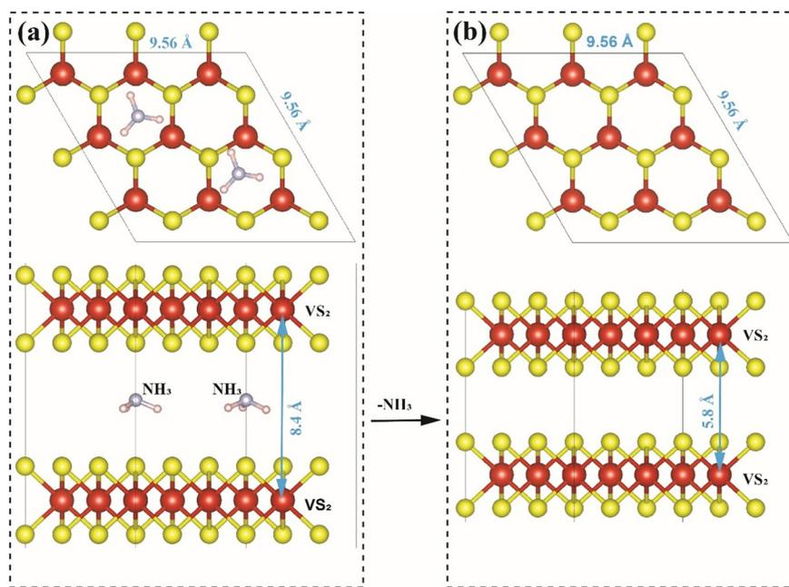
Fig. 9 Top and side view of two VS<sub>2</sub> sheets in the (a) presence and (b) absence of two intercalated ammonia molecules, indicating that the presence of ammonia increases the *d* spacing between VS<sub>2</sub> sheets.
