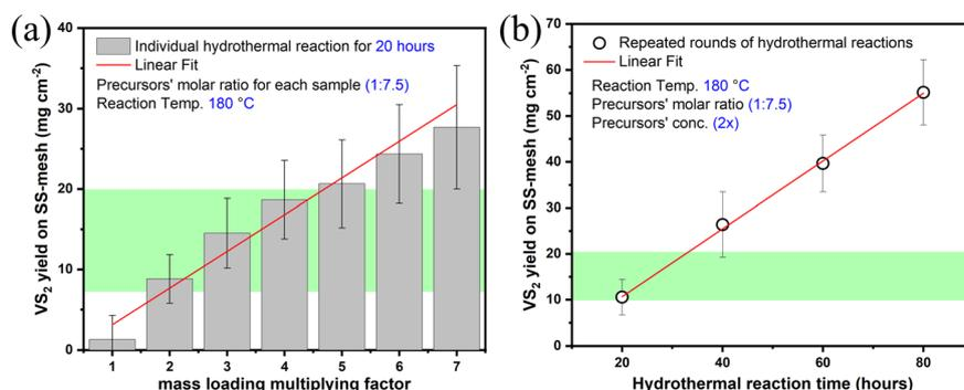
Fig. 4 (a) Bar chart displaying the effect of initial precursors' ( $\text{NH}_4\text{VO}_3$ :TAA) mass loadings (each bar has fix ratio of 1:7.5 times multiplying factor) on the  $\text{VS}_2$  yield after a single-step hydrothermal process for 20 hours of reaction time. (b) Scattered chart of a sample (1:7.5 mmol  $\times$  2) showing the effect of repeated rounds of hydrothermal reactions, of 20 hours each, on the  $\text{VS}_2$  yield.
