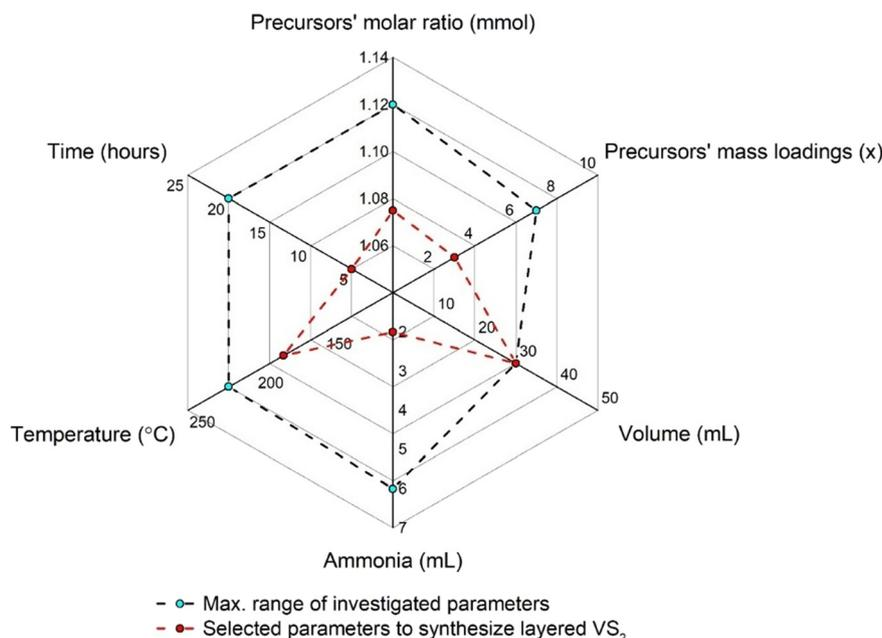
Fig. 11 Radar chart summarizing the investigated reaction parameters and the optimized conditions for layered VS<sub>2</sub> synthesis.
