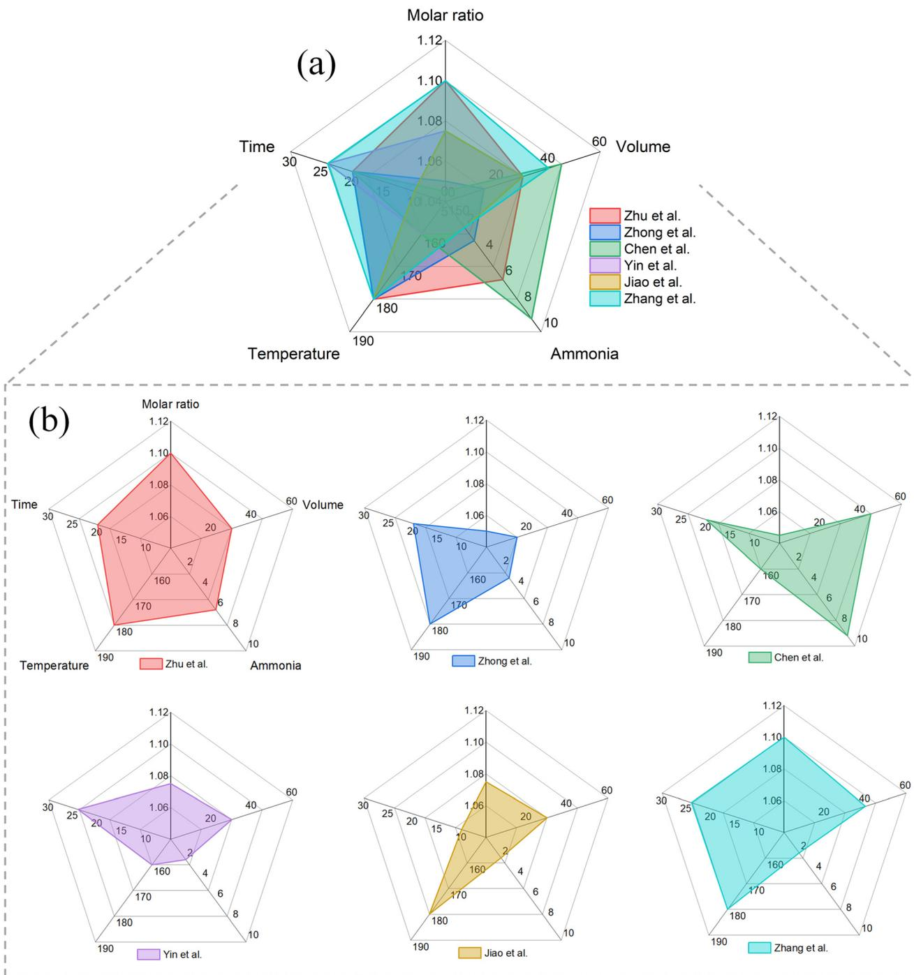
Fig. 1 (a) Radar chart showing the reaction variables used in the literature: molar ratio (%), volume (mL), amount of ammonia (mL), reaction temperature ( $^{\circ}\text{C}$ ), and time (hours). (b) Expansion of Fig. 1a to represent the individual study.
