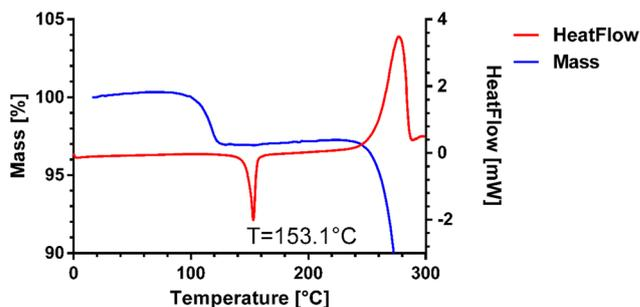
Fig. 3 DSC and TGA of venetoclax acetonitrile solvate.
