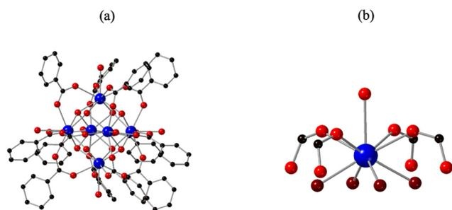
**Fig. 1** Illustration of (a) **Th<sub>6</sub>** cluster and (b) the local coordination environment about the Th metal centers. Thorium and carbon are shown in blue and black respectively. Oxygen atoms in water and the benzoate ligands are shown in red, and μ<sub>3</sub>-oxygens in maroon. Hydrogen atoms and disorder have been omitted for clarity.
