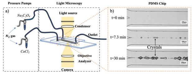
Fig. 1 a) The experimental setup with a microfluidic platform consisting of a pressure pump, a light source and a microscope with the chip.  $CaCl_2$  and  $Na_2C_2O_4$  were dissolved in artificial urine. b) The images were taken under the same experiment conditions (experiment AU4) at three timelapses of 0, 7.3 and 30 minutes after the first crystal emerged.
