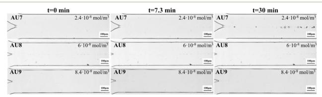
Fig. 6 Microscopy images of the microfluidic channel for experiments AU7, AU8 and AU9 (different rows) with different amounts of OPN;  $2.4 \times 10^{-8}$  mol m<sup>-3</sup>,  $6.0 \times 10^{-8}$  mol m<sup>-3</sup> and  $8.4 \times 10^{-8}$  mol m<sup>-3</sup>, respectively, at a fixed Ca: Ox molar ratio of 7.5 and a flow velocity of 0.015 m s<sup>-1</sup>. Three time lapses after the first appearance of crystals (in columns) with a 10× objective with a 100  $\mu$ m scale bar.
