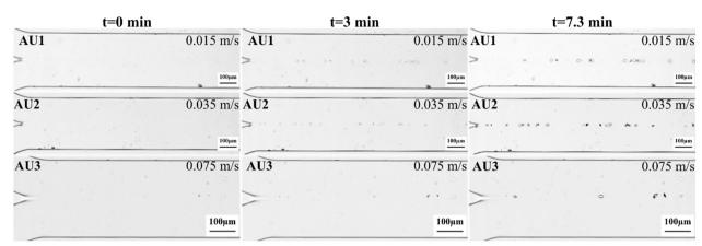
Fig. 4 Microscopy images of the microfluidic channel for three experiments AU1, AU2 and AU3 (different rows) for varying flow velocities at 0.015, 0.035 and 0.075 m s<sup>-1</sup>, respectively, at a fixed Ca: Ox molar ratio of 7.5. Time lapses of 0, 3 and 7.3 minutes after the first appearance of crystals (in columns) with a  $10^{\circ}$  objective, except for AU3 (with a  $20^{\circ}$  objective) with a 100  $\mu m$  scale bar.
