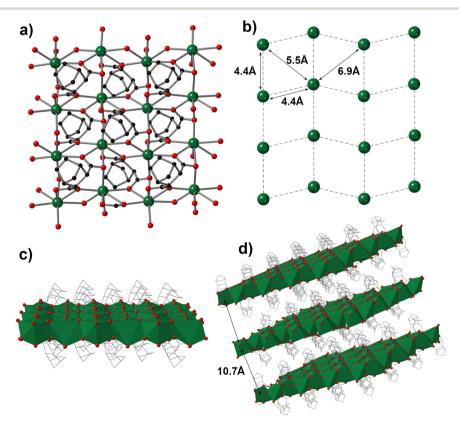
Fig. 1 (a) A portion of the 2D sheet structure of 1. (b) Illustration of the (4,4) network topology in 1 with various metal-to-metal distances. (c) Perspective view of the single 2D layer. (d) Perspective view of the three 2D layers in 1. The distance between the two adjacent layers is 10.7 Å.
