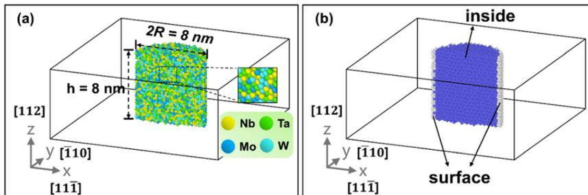
Fig. 1 Atomic configuration and cross-section of the NbMoTaW RHEA nanowire with a radius ( $R$ ) of 4 nm and the loading direction of [112]. (a) Cross-section with atoms colored by the element type. (b) Cross-section with atoms colored by the local structure, with blue and white balls denoting inner and surface layer atoms, respectively.
