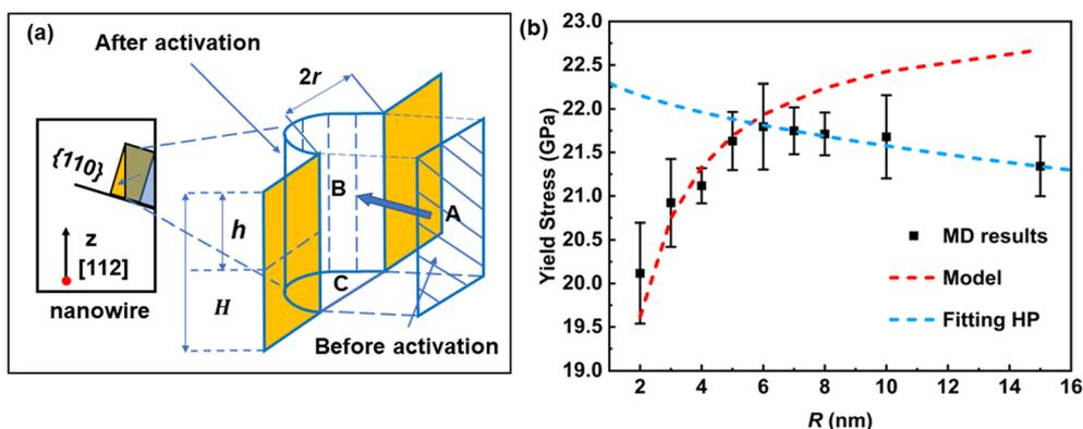
Fig. 5 (a) Schematic of dislocation activation from the surface of the nanowire (orange plane). (b) Comparison of yield stresses of NbMoTaW nanowire samples with different  $R$  obtained using theoretical model predictions [red curve, eqn (7) for the IHP stage; blue curve, fitting curve using the HP relation] with that simulated using MD (black points).
