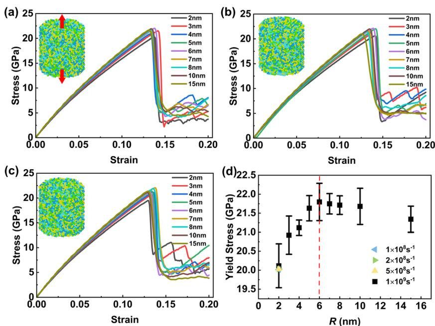
Fig. 2 (a)–(c) Stress–strain curves of sample groups A, B, and C with different  $R$ . (d) Variation of yield stress with  $R$ , revealing a transition from the HP relation to the IHP relation at  $R = 6$  nm. Simulations on sample group A with  $R = 2$  nm at different strain rates confirm that the deviation of the yield stress obtained with different strain rates remains within the error range.
