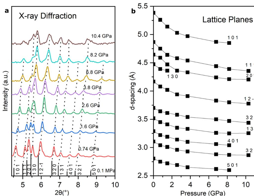
Fig. 4 (a) Selected synchrotron X-ray diffraction patterns as a function of pressure with major peaks labeled. Six principal peaks indexed with  $hkl$  values 111, 201, 12-1, 320, 131, and 321 are observed. (b) The  $d$ -spacing values obtained from the X-ray diffraction data are labeled with their Miller indices. The continuous decrease in  $d$ -spacings indicates no major change in the hexagonal structure on compression.
