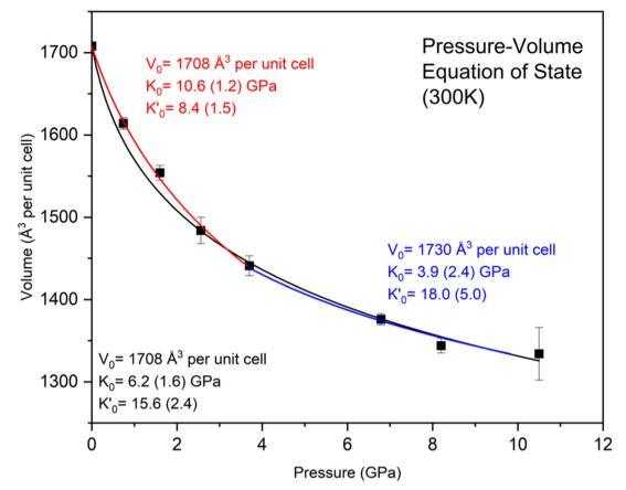
Fig. 6 P-V relations of 2,3-diphenyl-2H-azirine obtained from the X-ray diffraction. The black solid line shows a Vinet EOS fit of the entire data set, while the red line indicates the fit from ambient to 3.7 GPa, and the blue line shows the fit from 3.7 GPa to 10.5 GPa. The P-V data are listed in Table S2:
