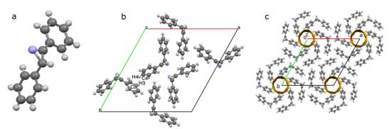
Fig. 1 (a) 2,3 Diphenyl-2*H*-azirine molecule. (b) Unit cell structure viewed along the *c*-direction, showing the distance between the C4B-H4B and C3A-H3A molecules (see text). (c) Expanded view of the structure along the c-axis showing the voids in the unit cell.
