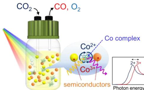
**Direct observation of an ionic cobalt complex electron mediator via *operando* X-ray absorption spectroscopy in photocatalytic Z-scheme CO<sub>2</sub> reduction with (CuGa)<sub>0.3</sub>Zn<sub>1.4</sub>S<sub>2</sub> and BiVO<sub>4</sub>**
