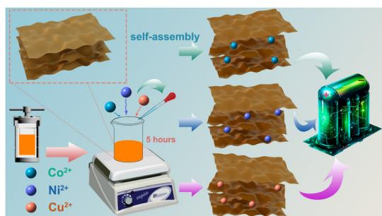
**Divalent transition metal ion intercalated hydrated V<sub>2</sub>O<sub>5</sub> nanosheet cathodes for ultra-long cycling aqueous zinc-ion batteries**
