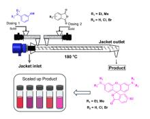
Continuous flow solvent-free and catalyst-free mechanochemical production of rhodamine B dyes and their derivatives
