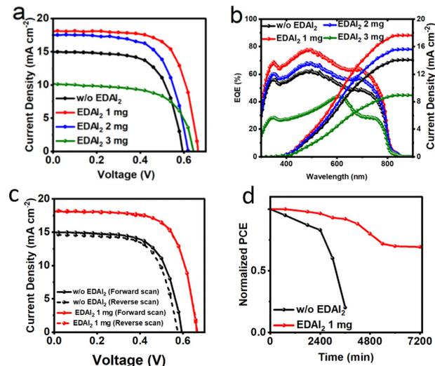
Fig. 4 (a) Forward-scan current density-voltage ( $J$ - $V$ ) curves of the devices without and with various amounts of EDAl<sub>2</sub>. (b) EQE curves. (c)  $J$ - $V$  curves of the control and 1 mg mL<sup>-1</sup> EDAl<sub>2</sub>-based solar cells measured in the forward and reverse scan directions. (d) Normalized PCE stability of the devices measured outside an inert environment.
