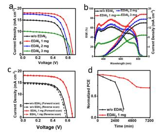
Fig. 4 (a) Forward-scan current density-voltage (J-V) curves of the devices without and with various amounts of EDAI2. (b) EQE curves. (c) J-V curves of the control and 1 mg mL<sup>-1</sup> EDAl<sub>2</sub>-based solar cells measured in the forward and reverse scan directions. (d) Normalized PCE stability of the devices measured outside an inert environment.
