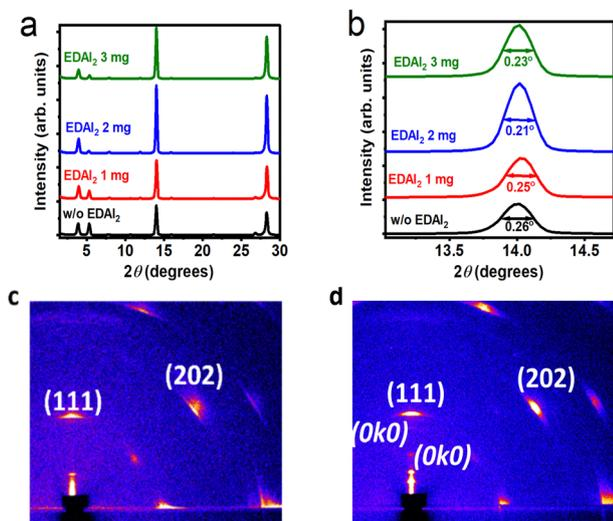
Fig. 1 (a) XRD patterns for PEA<sub>2</sub>FA<sub>6</sub>Sn<sub>7</sub>I<sub>15.4</sub>Br<sub>6.6</sub> films with different amounts of EDAI<sub>2</sub> and (b) an extraction of the peak around 14.0° for calculation of the full-width at half-maximum. GIWAXS images of (c) the control film and (d) a film with 1 mg mL<sup>-1</sup> EDAI<sub>2</sub>, acquired at an incidence angle of 0.5°.
