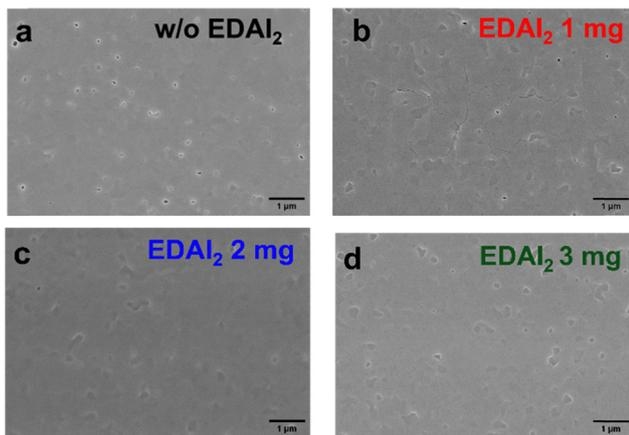
Fig. 2 SEM images of (a) a control film and films containing (b) 1 mg mL<sup>-1</sup>, (c) 2 mg mL<sup>-1</sup>, and (d) 3 mg mL<sup>-1</sup> of EDAl<sub>2</sub>.
