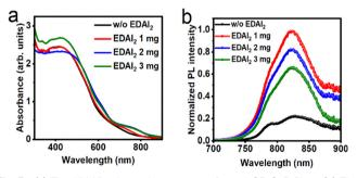
Fig. 3 (a) The UV-Vis absorption spectra of quasi-2D SnP films. (b) The photoluminescence spectra of the deposited SnP films, acquired at an excitation wavelength of 525 nm.
