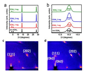
Fig. 1 (a) XRD patterns for  $PEA_2FA_6Sn_7I_{15.4}Br_{6.6}$  films with different amounts of  $EDAl_2$  and (b) an extraction of the peak around  $14.0^{\circ}$  for calculation of the full-width at half-maximum. GIWAXS images of (c) the control film and (d) a film with 1 mg mL<sup>-1</sup> EDAI<sub>2</sub>, acquired at an incidence
