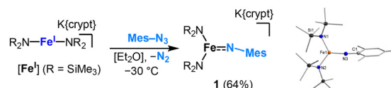
Scheme 1 Left: Synthesis of \text{K}\{\text{crypt}\}[\text{Fe}(\text{NMe}_3)(\text{NR}_2)_2] , 1 . Right: Molecular structure of the complex anion of 1 (ellipsoids shown at a 50% probability). H atoms are omitted for clarity. Important bond lengths (Å) and angles (°): Fe1–N1 1.945(2), Fe1–N2 1.963(2), Fe1–N3 1.753(2), N3–C Aryl 1.337(2), N1–Fe1–N2 118.08(4), Fe1–N3–C Aryl 173.04(1).
